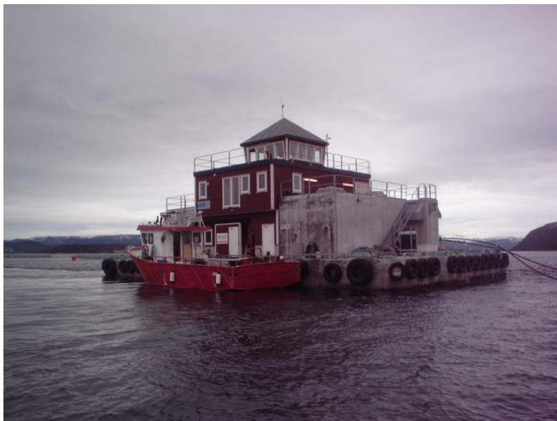
Figure 1-Feeding Barge of concrete (Marine-Construction 2016)
