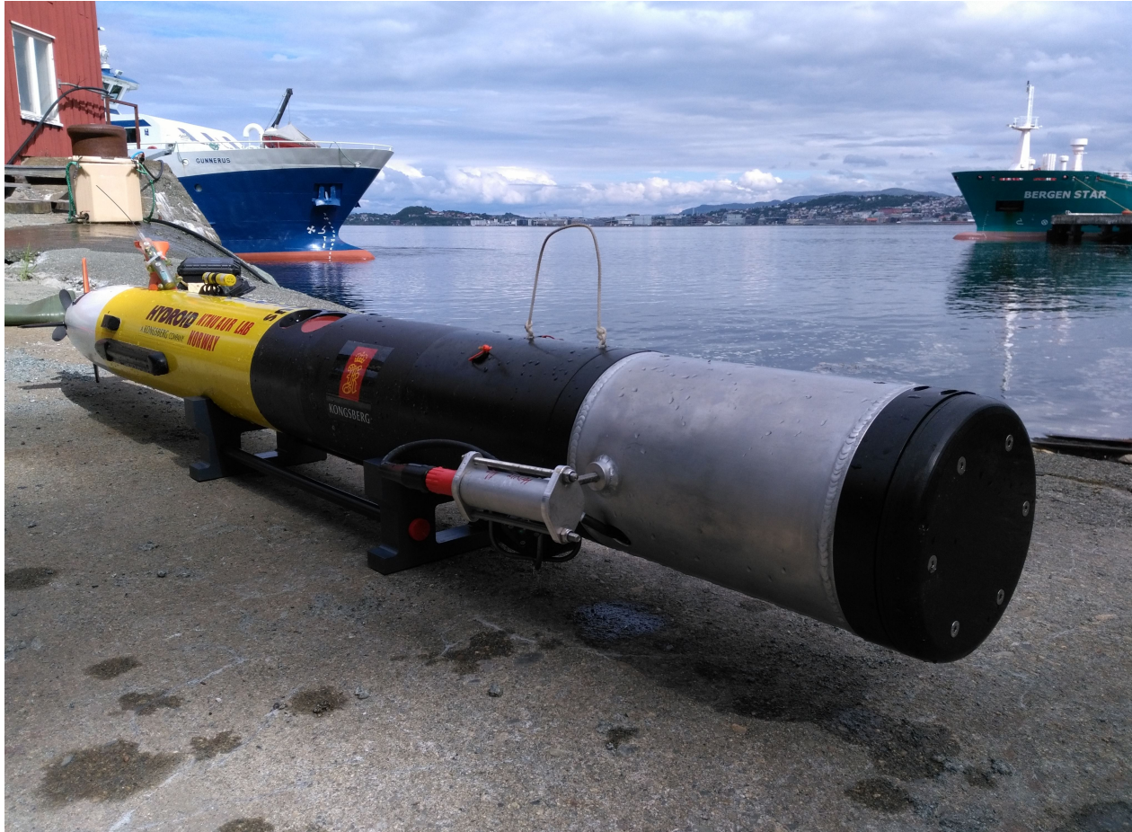
Figure 6.7: Remus with the installed magnetometer housing
