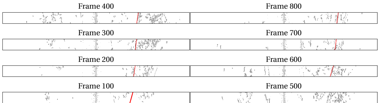
Figure 7.3: A selection of edge images with the detected line drawn in red
