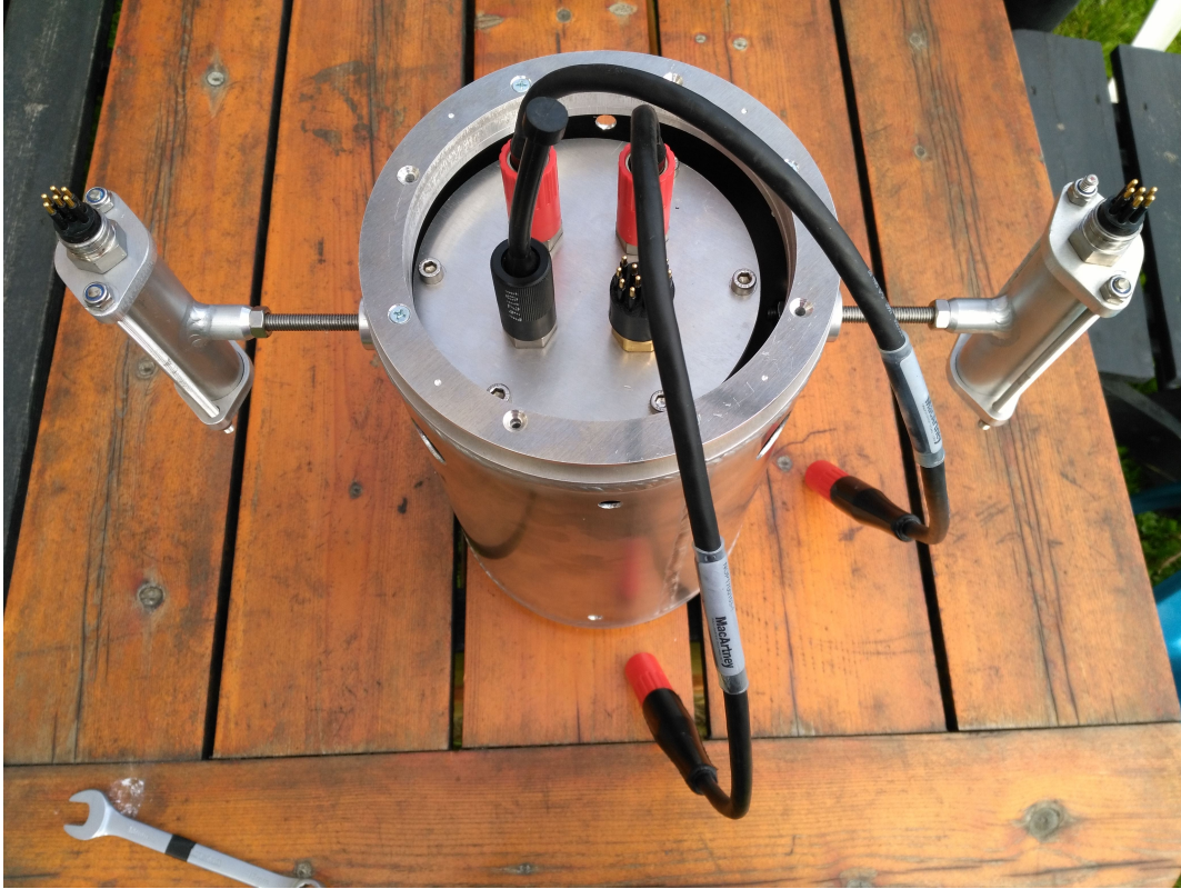
Figure 6.6: Housing with the magnetometers placed on the outside. A Raspberry PI is placed in the dry section in the middle
