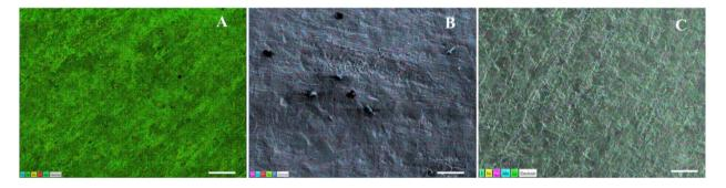
Fig. 4. EDS mapping of cylinder surfaces after 5 weeks at stripper conditions for (A) 30 wt% MEA solution, (B) 30 wt% MEA with 1 wt% bicine, and (C) 30 wt% MEA with 1 wt% HeGly. Scale bars denote 100 µm.
