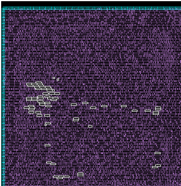
Figure 6.8: Placement of flip-flops cells without relative placement directives
