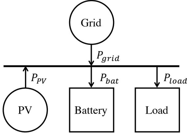
**Figure 3.1:** Schematic of the household with indicated power directions.
