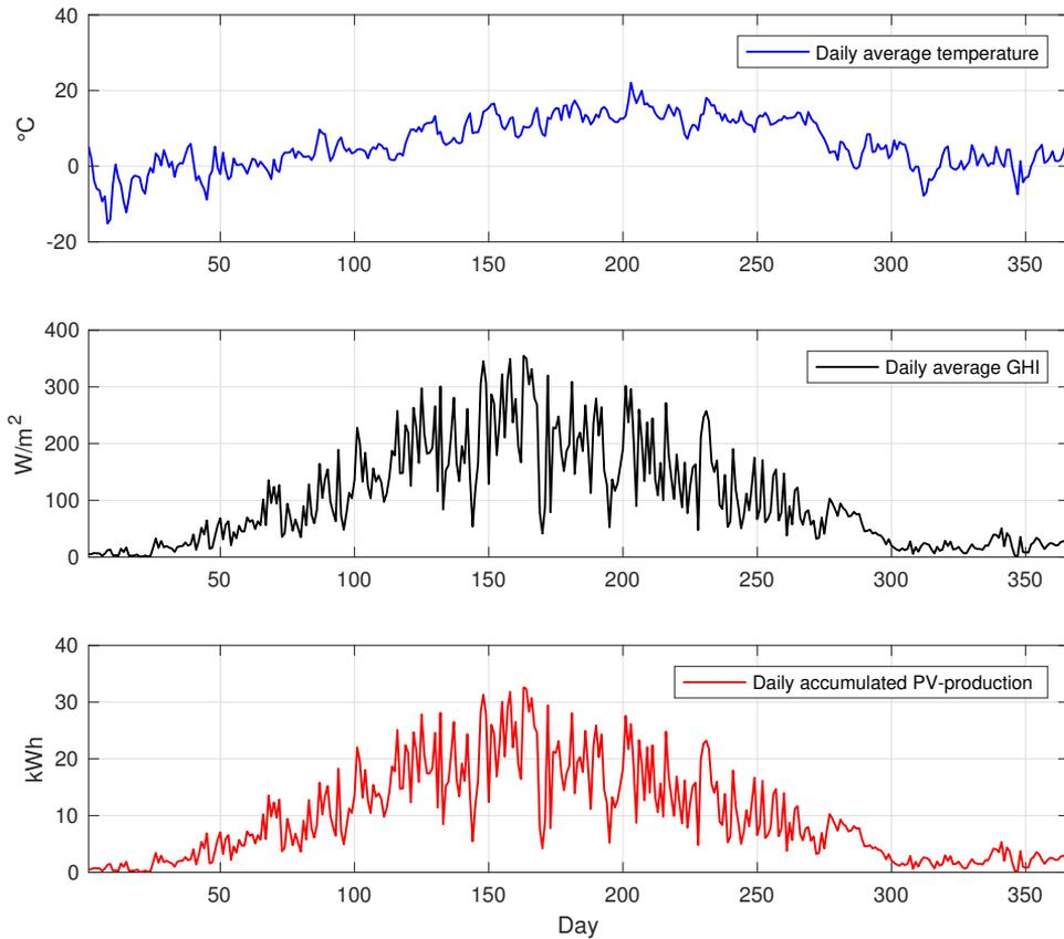
**Figure 4.4:** Plot of daily average temperature (upper plot) and irradiance (middle plot) in 2016, and the resulting accumulated PV-production.
