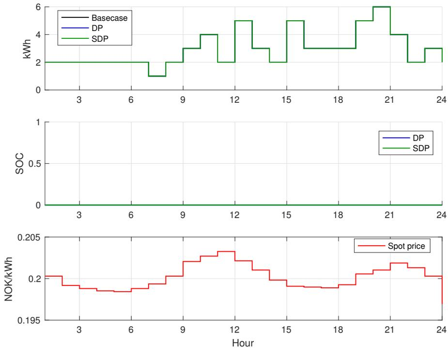
**Figure 5.9:** Saturday the 16th of April 2016, standard settings without PV under the energy based UT. Upper plot shows  $P_{grid}$  for the basecase, DP and SDP. Middle plot shows the SOC of the battery. Lower plot shows spot price.
