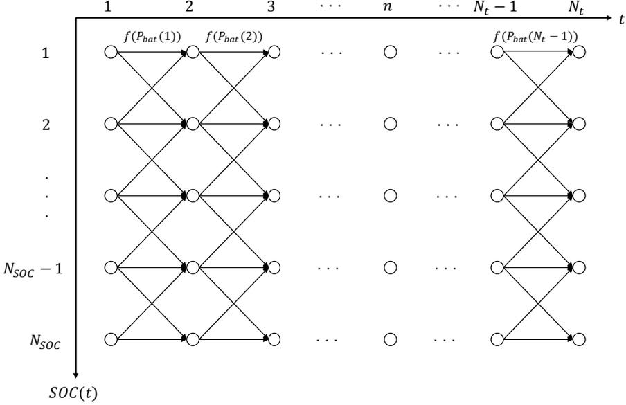
**Figure 2.1:** Illustration of a DP problem with  $N_t$  time steps and  $N_{SOC}$  states of SOC.
