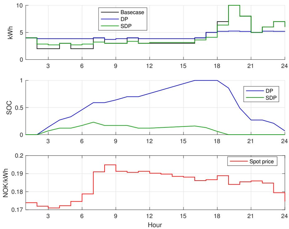
**Figure 5.12:** Friday the 12th of February 2016, standard settings without PV under the power based UT. Upper plot shows  $P_{grid}$  for the basecase, DP and SDP. Middle plot shows the SOC of the battery. Lower plot shows spot price.
