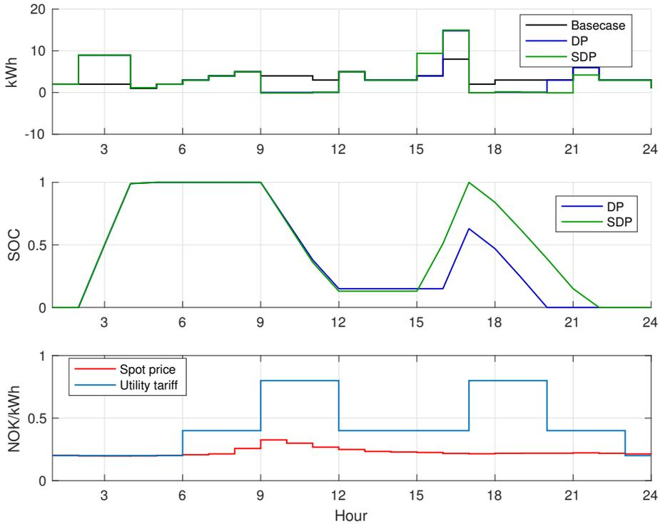
**Figure 5.10:** Wednesday the 13th of April 2016, standard settings without PV under the time based UT. Upper plot shows  $P_{grid}$  for the basecase, DP and SDP. Middle plot shows the SOC of the battery. Lower plot shows spot price and UT.
