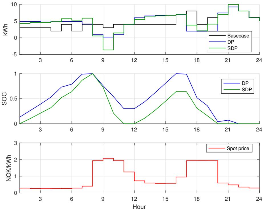
**Figure 5.11:** Thursday the 21st of January 2016, standard settings without PV under the power based UT. Upper plot shows  $P_{grid}$  for the basecase, DP and SDP. Middle plot shows the SOC of the battery. Lower plot shows spot price.
