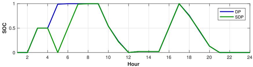
**Figure 5.6:** Resulting SOC from the DP- and SDP-optimisation of load 3 for Wednesday the 20st of January of 2016. Standard settings under the time based UT.
