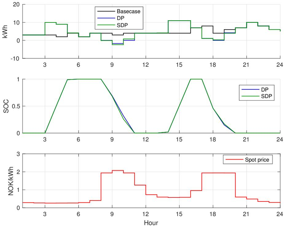
**Figure 5.8:** Thursday the 21st of January 2016, standard settings without PV under the energy based UT. Upper plot shows  $P_{grid}$  for the basecase, DP and SDP. Middle plot shows the SOC of the battery. Lower plot shows spot price.
