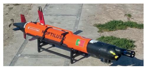
Figure 6.8: Light autonomous underwater vehicle (LAUV).
