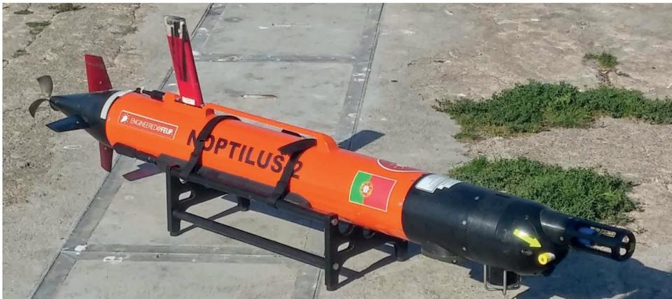
Figure 6.8: Light autonomous underwater vehicle (LAUV).
