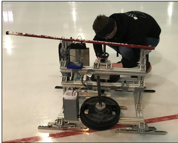
Figure 4: The tribometer on the ice during assembly. The tribometer is supported by five skates, where the skate in the middle is attached to the steel bridge and loading cell. The battery used to power to the instruments is in the square grey box on the left in the picture. The blue computer on top of the tribometer controls the photocells.
