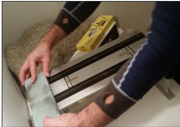
Figure 7: The whetstone in the picture is the first one to be used when preparing skate blades, a very coarse grade. The whetstone would slide back and forth until a satisfactory finish is met. Water is the most common lubricant when grinding the steel blade, this is applied by adding a few drops on the surface of the whetstone.
