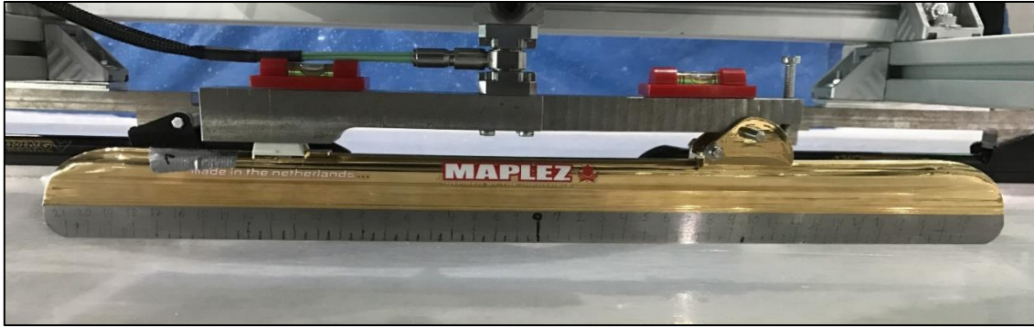
Figure 14: The picture illustrates how the contact surface could be measured when applying load to the blade. A thin paper would slide under the skate steel from both sides. When the papersheet stopped, the distance from center of the blade would be noted and calculated to a nominal contact length. Pressure from the skate on the ice was calculated from known values of length, width and load on the skate.
