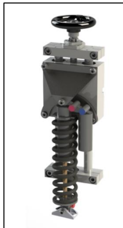
Figure 6: A graphic presentation of the manual actuator with the shock absorber used for the tribometer. The actuator was mounted to the aluminium beams on the tribometer, in the centre of gravity. Loading and offloading of the skate blade was done by turning the wheel on the top [4].
