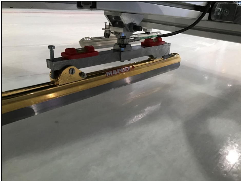
Figure 5: The steel bridge was installed with two levelers, one on each side, to set a null point prior to loading the skate. The bridge is connected to the loading cell with four bolts, and is parallel to the direction of movement. The connection points to the skate blade are like that of a real speed skating shoe. This is a static connection, with no room for movement.
