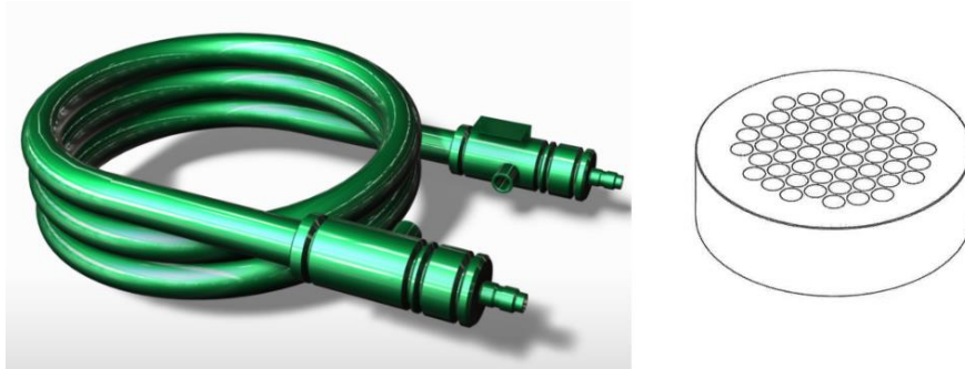
Figure 31. Schematic of a coaxial heat exchanger. The cross-section is shown to the right.
