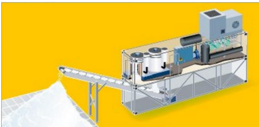
Figure 16. Schematic of the model SF220 from TechnoAlpin AG
