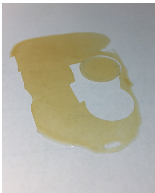
Figure A.5: PTMSP/ZIF-8L membrane made with casting knife.
