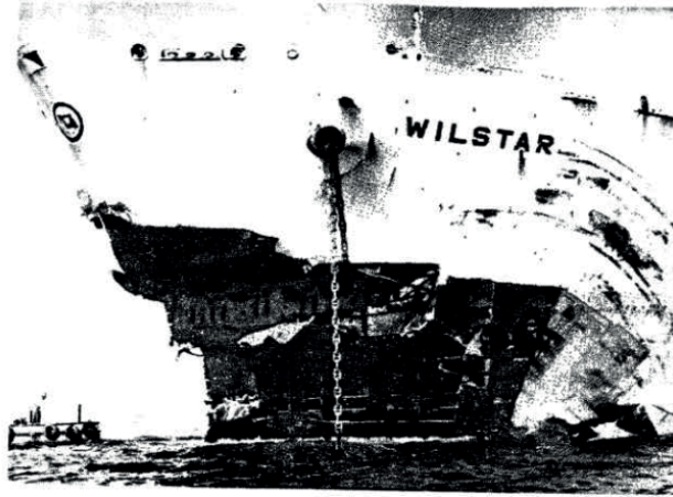
Figure 1.1: A picture of the tanker damaged by encountering an advancing giant wave when going in the Agulhas Current on May. 17, 1974, from [7].
