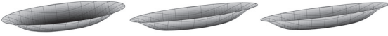
Figure 3: Super-Gaussian model ship pressure distributions from Eq. (21). Aspect ratios (left to right) W = 3, 5, 8 .
