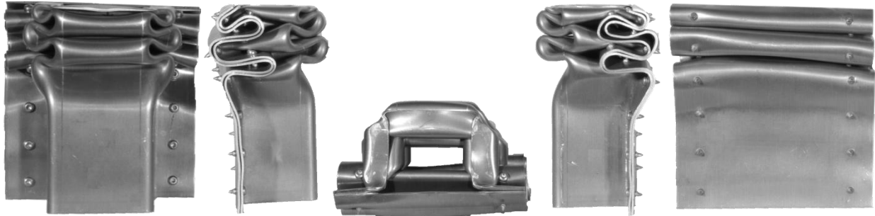
Fig. 16: Deformed single-hat section from dynamic axial crushing test, viewed from different directions.
