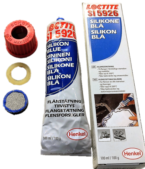
Figure 4.2: Application of blue silicon gel onto a thermally sprayed sample, creating an extra barrier against leakage.
