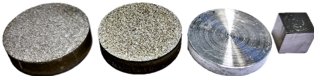
Figure 4.1: Front side of test samples - Left : DSA sample, 2nd Left : TSA sample, 2nd Right : Anode sample, Right : CS-cube.
