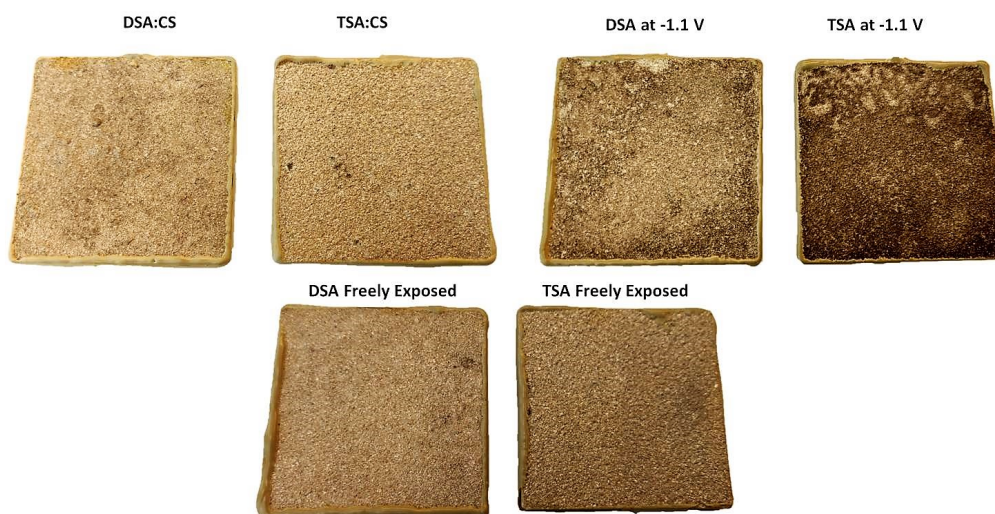
Figure 8.4: Samples embedded in mud after cleaning in Nitric Acid.
