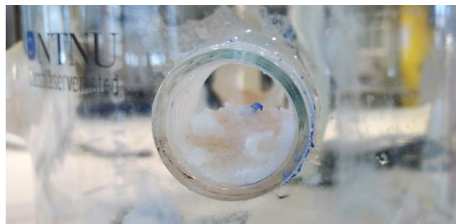
Figure 7.3: Corrosion products in the protruding part of 80°C container, where the coupled DSA sample was attached.
