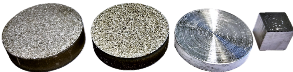
Figure 7.1: Initial surface conditions of test samples - Left : DSA sample, 2nd Left : TSA sample, 2nd Right : Anode sample, Right : CS-cube.
