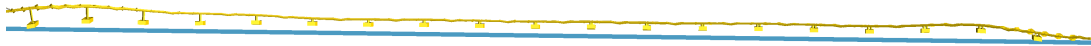
Figure 8.47: Bridge shape at maximum vertical displacement for fully correlated swell from west. Displacements scaled with a factor of 100.
