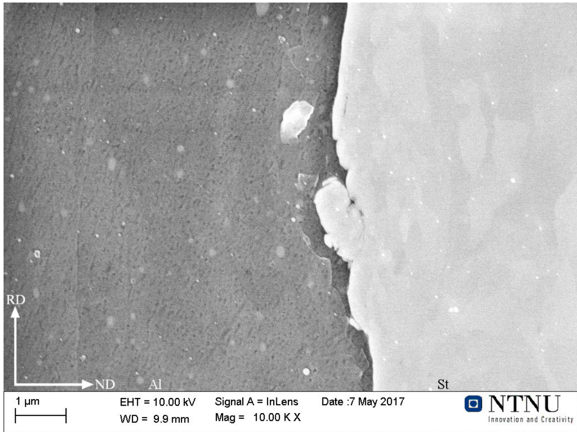
Figure 52: SAB-200 at 10.000X, with aluminum on the left and steel on the right. A large steel fragment is seen at the CRB bond, as well as a large particle embedded in the aluminum surface. Cracks are seen underneath the steel surface, following in the direction of rolling.
