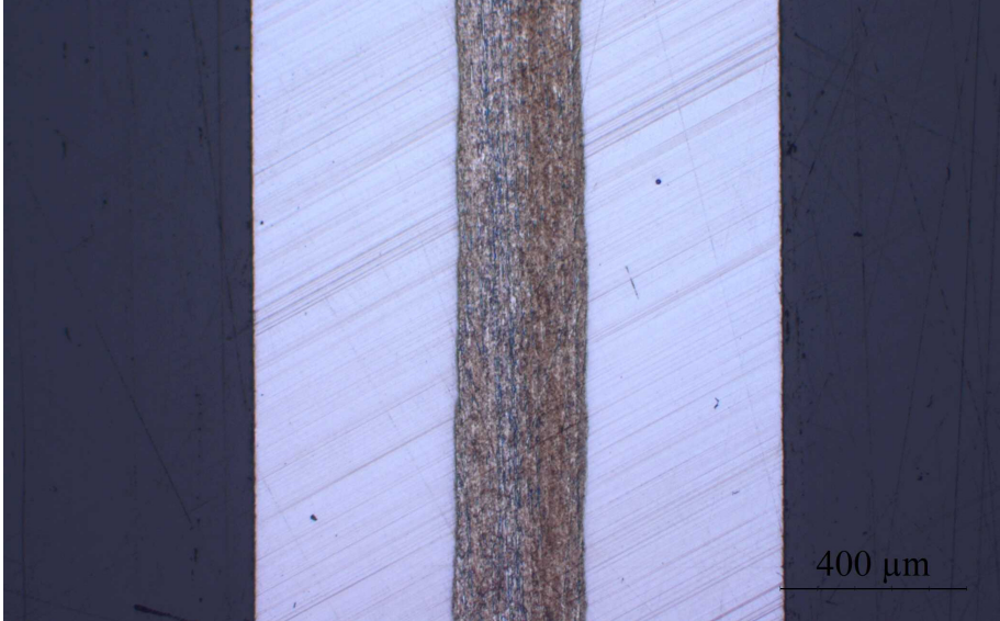
Figure 61: BSA-150 at 50X. The aluminum was reduced to 0,28 mm, while the steel was reduced to an average of 0,43 mm, giving a percent reduction of 69 % and 57 %, respectively.
