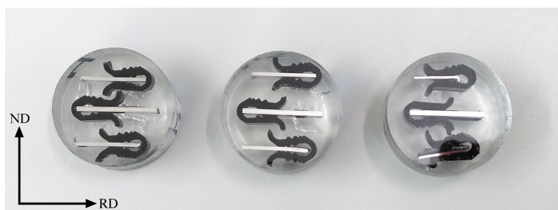
Figure 14: Three of the finished microstructural samples. The section at the center of each sample is the actual CRB specimen, while the outer pieces are IF steel meant to stabilize the samples during grinding and polishing. The black plastic clips were used to hold each sheet in place during epoxy casting.
