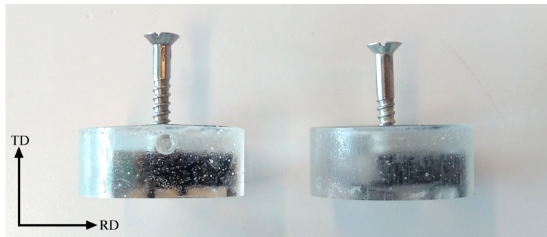
Figure 15: Two samples prepared for anodizing. A wooden screw was inserted from the back of each sample, contacting the specimen to be anodized. This ensured that electric contact could be achieved with the specimen, required for anodizing to take place.
