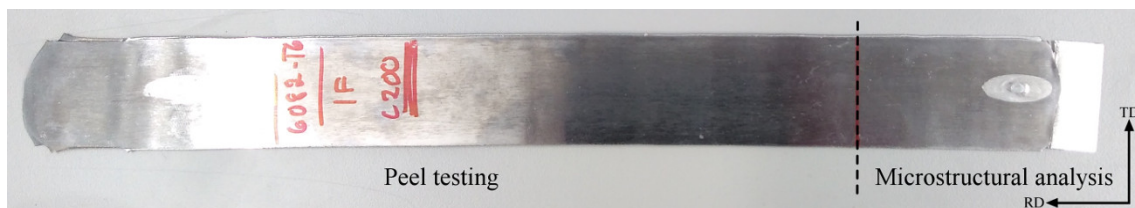
Figure 13: A completed sheet of cold roll bonded IF steel and AA6082 aluminum, with a relatively large thickness reduction, of 64 %. Flattened rivets can be seen on either end of the sample, as well as the aluminum sheet sticking out on the right side.
