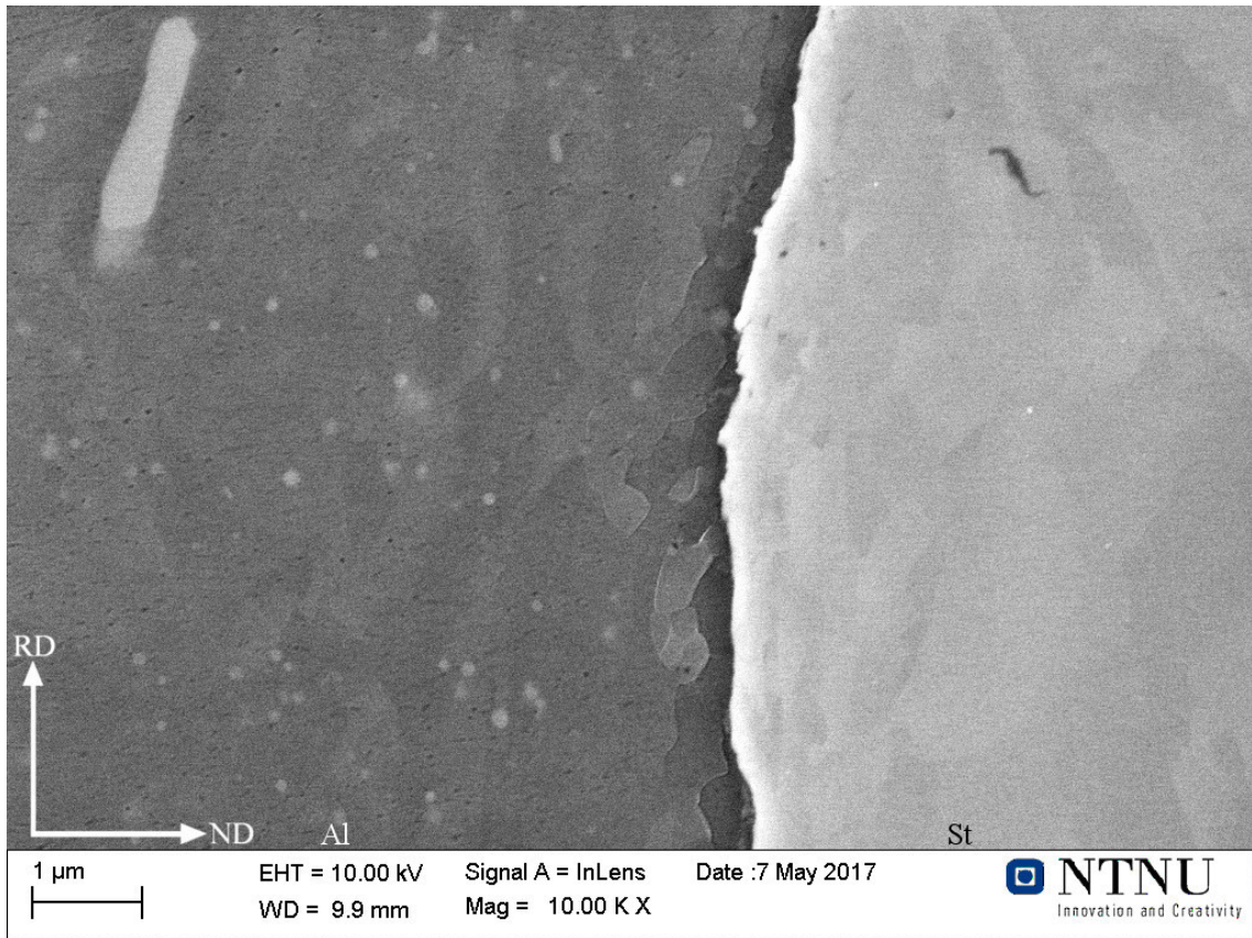
Figure 44: SBA-200 at 10.000X, with aluminum on the left and steel on the right. Several jagged edges are seen sticking out from the steel side of the interface, which may be pieces of the fractured oxide layer. A few grains are visible in the aluminum, as well as several particles.
