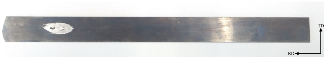
Figure 17: One of the finished peel testing samples. The sample has been machined down to a width of 20 mm, and a length of approximately 250 mm. A flattened rivet is visible on the left side of the sample.
