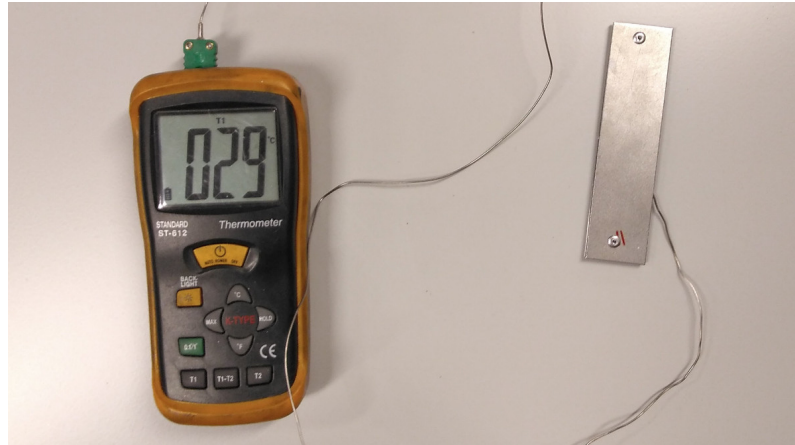
Figure 11: A thermometer used to calibrate the oven. The k-sensor is locked in place between two of the sheets in a three layered dummy CRB sample, as close to the center of the sample as possible. The required time for CRB samples to reach their pre-heat temperature could thus be estimated.
