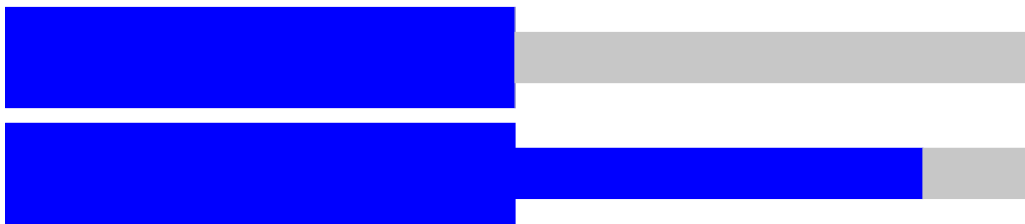
Figure 49: An incompressible slug moving from one cross sectional area into a four times smaller area. The top and bottom images correspond to times 0 and 0.1 seconds respectively. In the bottom image the slug front has moved a distance 0.4 m to the right.
