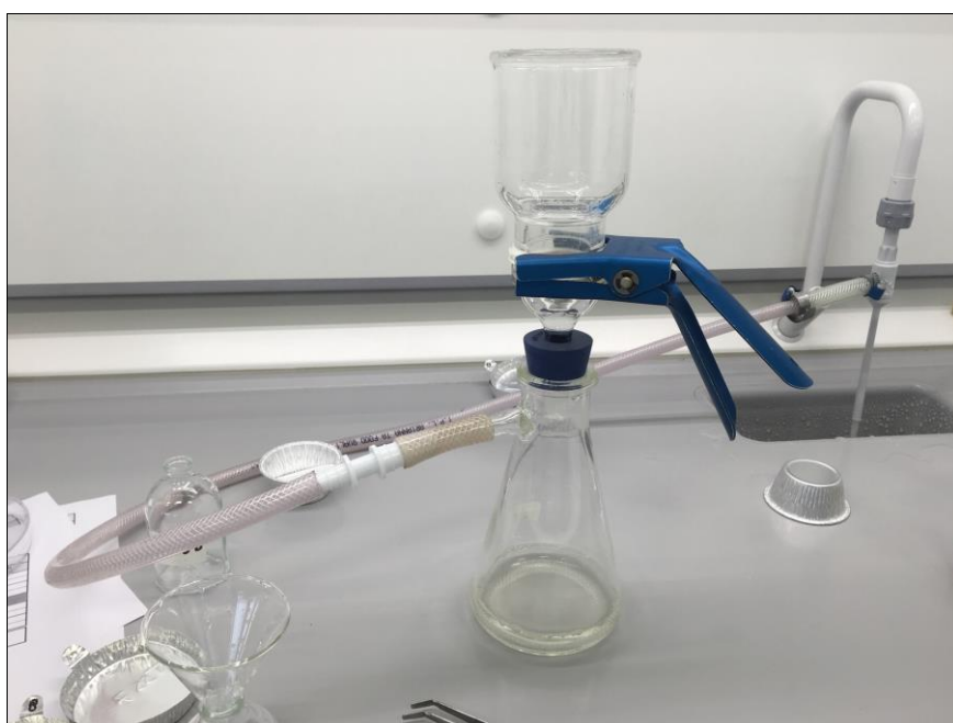
Figure 2.5. Experimental filtration setup for TDS, TSS and VSS analysis. Experiment was performed using suction filtration.
