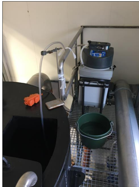
Figure 2.3. Set up for automatic sampler used for collecting fresh wastewater samples every two hours. Suction tube emerged in wastewater at all times.
