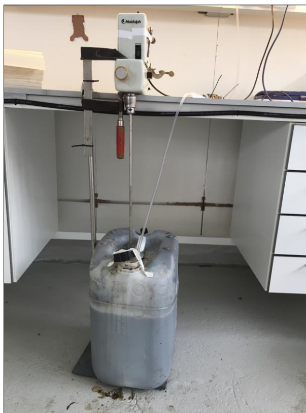
Figure 2.7. Experimental setup for maintenance of bio-P sludge during the experimental period. Mechanical mixer is emerged into container holding 25 L of bio-P sludge to prevent settling. Automatic timer is installed to ensure alternating anaerobic and aerobic conditions. Bio-P sludge is fed with acetate three times a day.
