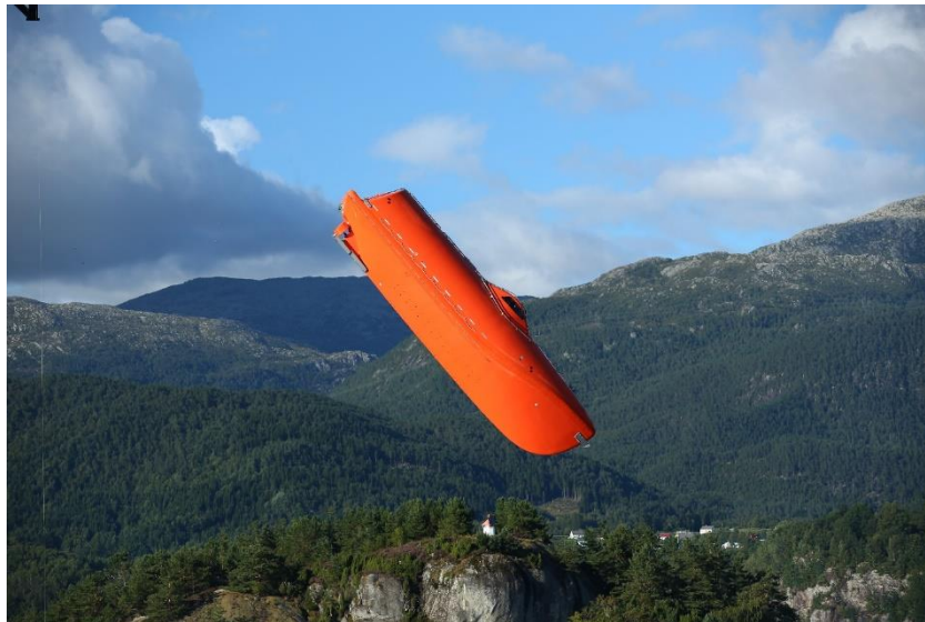
Figure 2.2: Shows a free-falling lifeboat in the free-falling phase. This is a Norsafe AS production, one of the leading lifeboat producers. (Consultance, 2017)
