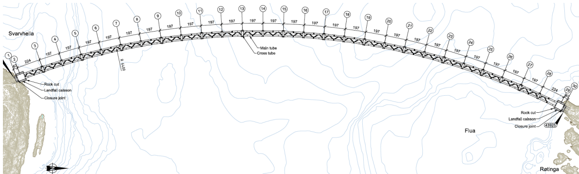
Figure 3.2: The horizontal alignment of the SFTB. The length of the bridge is arranged in a north-south orientation. The left side is the south end and the right side is the north end. Magnified figure in appendix A.1. (Reinertsen et al., 2016b).
