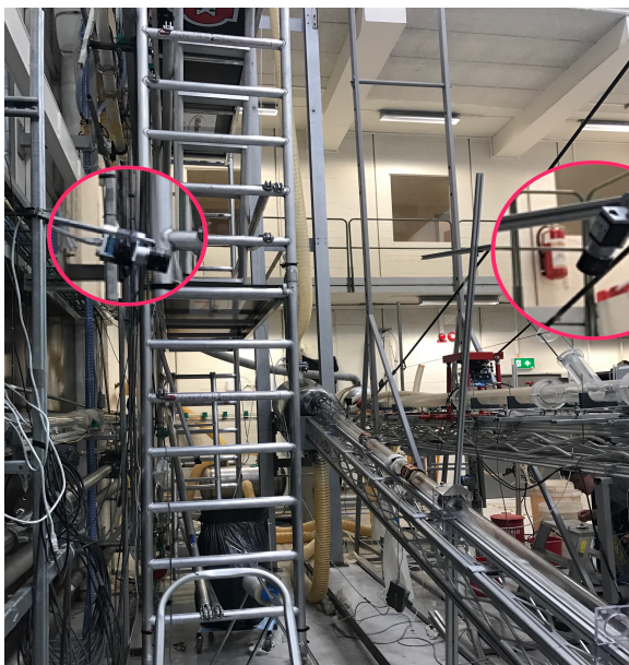
(a) Camera set up for inclination angles 25^\circ - 60^\circ .
