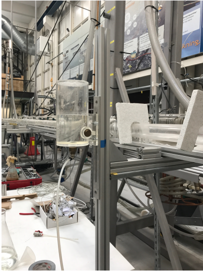
Figure 3.14: Set up for verification of static pressure with water.
