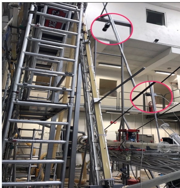
(b) Camera set up for inclination angles 70^\circ and 78^\circ .
