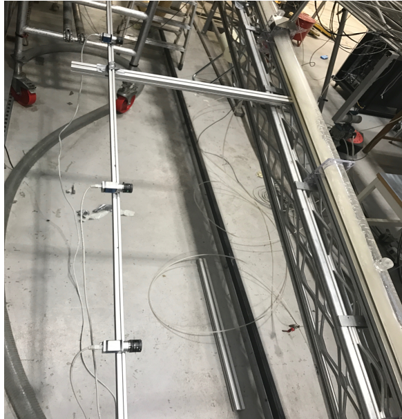
(b) Camera set up inclination angles 10^\circ - 20^\circ .
