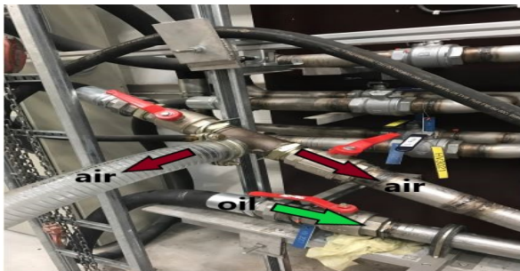
Figure 2: Mixture section before flexible pipe.
