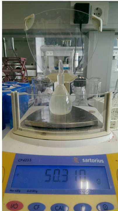
Figure 3.8: Density measurement using a picnometer.
