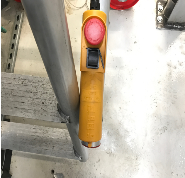
(a) Control device for changing pipe inclinations.
