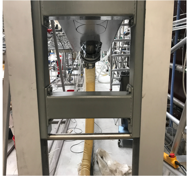
(b) Support beam for test section.
