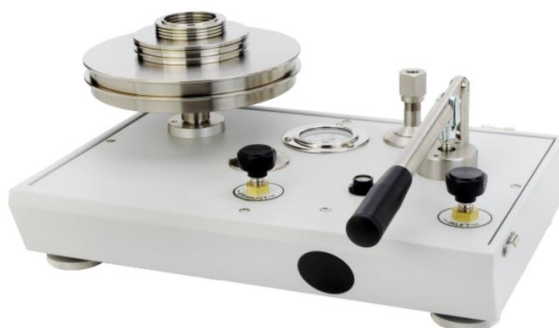
Figure 3.1: Deadweight manometer similar to the one at NTNU. Used for calibrating pressure transducers. Model: Fluke P3000 [36].
