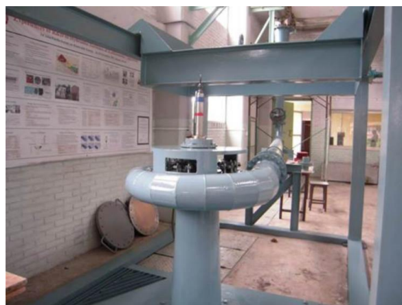
Figure 2.7: The simplified Francis turbine test rig at TTL. The rig was dismantled for maintenance when the writer visited KU in 20017. Photo: Biraj Sing Thapa.
