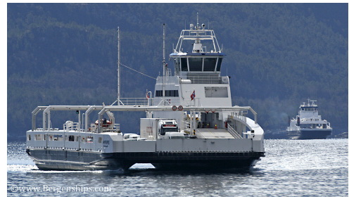
Figure 3: The electrically powered ferry between Oppedal and Lavik, Ampere .
