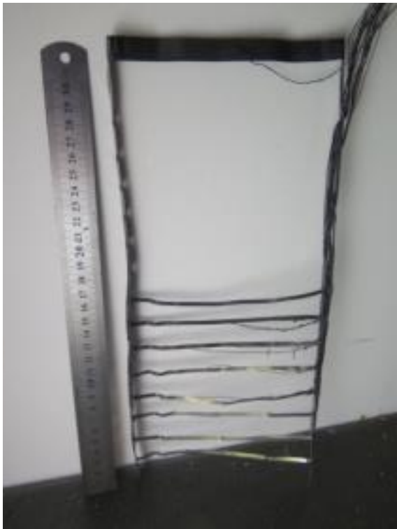
Figure 18: Picture of the thermocouple ladder. For comparison the ruler is 30 cm long.
