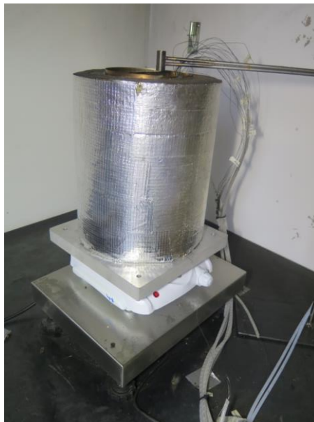
Figure 15: Test set up consisting of, from the bottom: scale, hotplate, aluminium plate, steel annulus and the insulated steel pipe.
