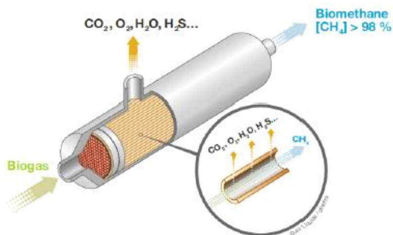
Figure 7: Process Flow Diagram of Membrane Separation (Bauer et al., 2013)
