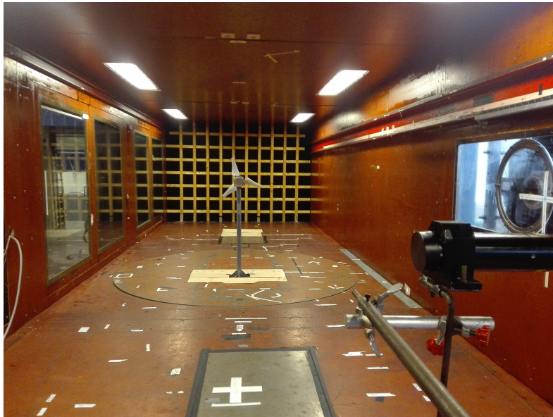
Figure 2: Picture of the test section with LDV probe mounted onto the traverse and the wind turbine and the grid installed.
