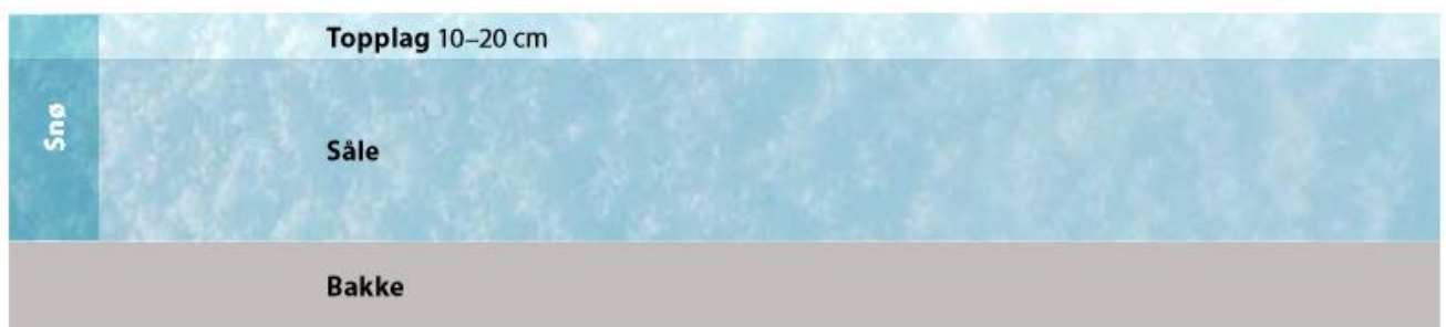
Figure 8 - Desired relationship between sole and top layer [5]
