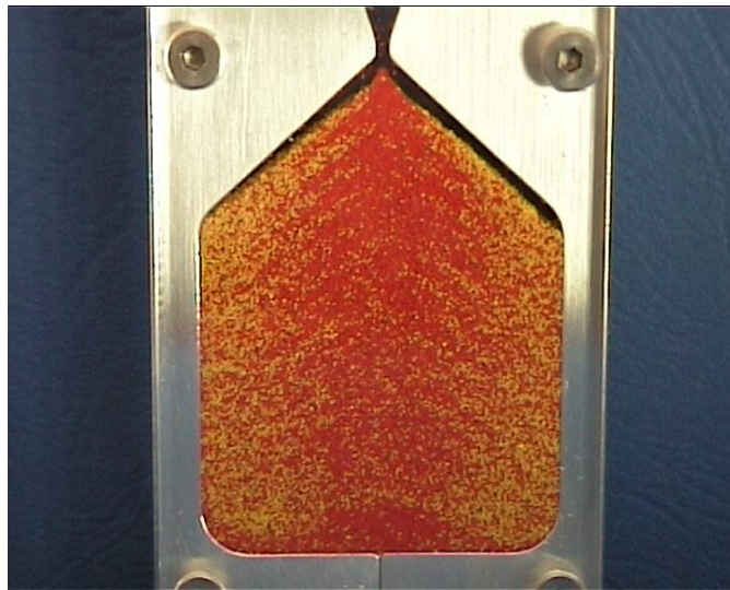
Figure 2.3: An example of segregation during filling due to particle size. The big particles are yellow, while the small particles are red [11].
