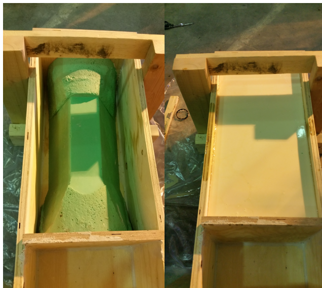
Figure 4.4: Creating the reproduced flume. Left: Box of plywood with negative imprint inside. Right: PUR poured and drying over the negative imprint to create the flume replica [Photo PPN]
