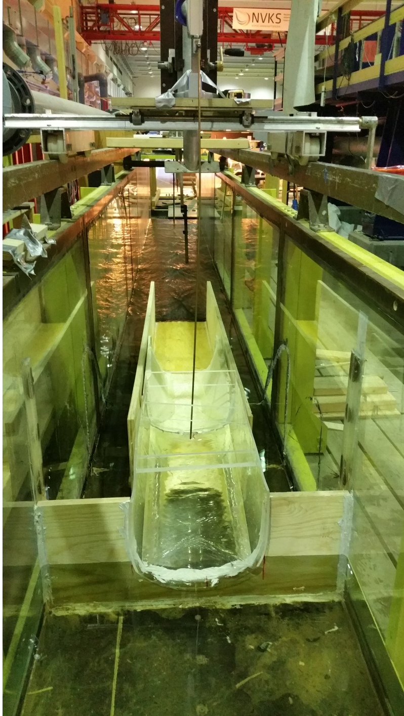
Figure 4.9: The model installed into the C-flume [Photo PPN]
