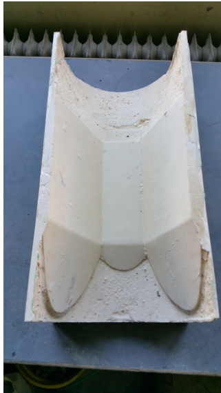
Figure 4.5: The reproduced Palmer-Bowlus flume from Risvollan [Photo PPN]
