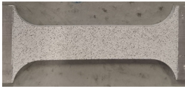
Figure 2.8: Test specimen with speckle pattern sprayed on.
