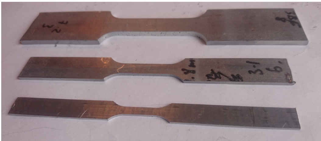
Figure 3.7: Dog bone specimens with thickness 1.0 mm, 1.8 mm and 3.3 mm.
