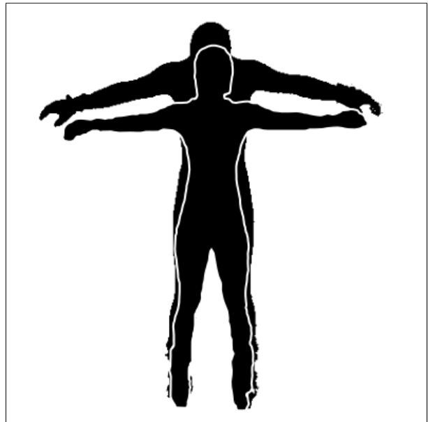
Figure 5.12: Visualization of the difference in frontal area of the smallest test subject, TS2 , and the biggest, TS6 , in the reference position.
