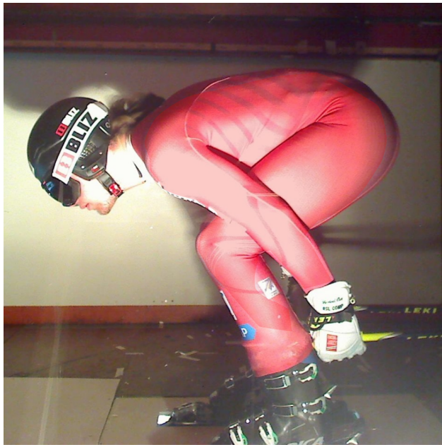
Figure 5.14: Side picture of TS6 in position 1, the flight position with the hands hidden behind the legs.
