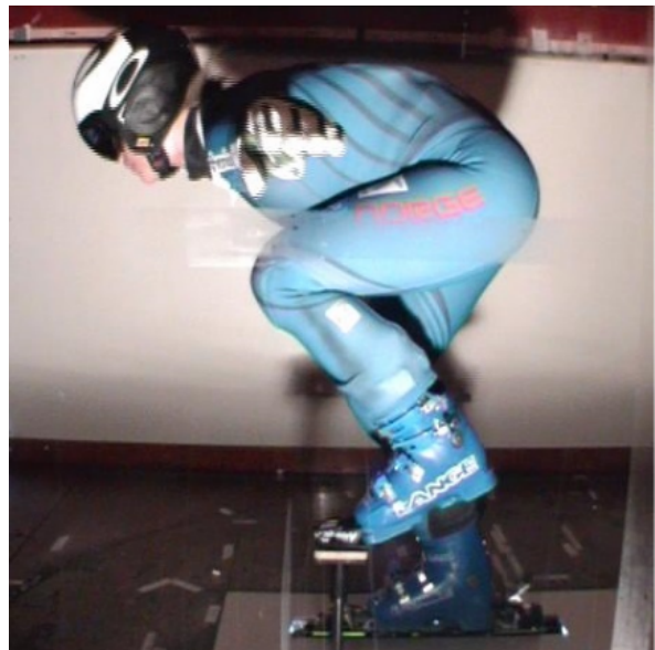
Figure 4.8: Measurement from the turning position experiment, with a low hip angle and the highest position tested for the left leg.
