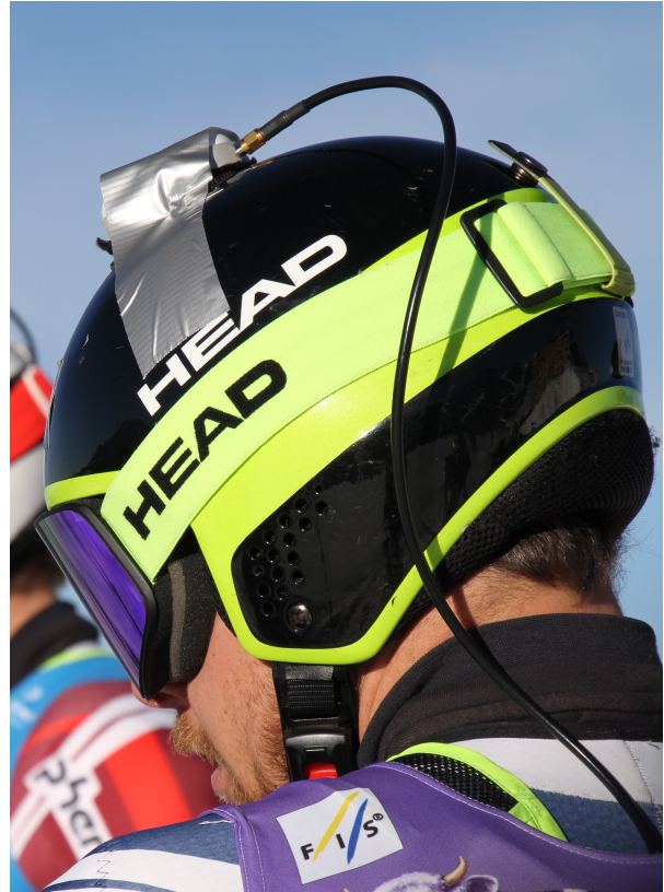
Figure 2.3: Skier with the antenna for the dGNSS mounted on the head. Foto: NSF
