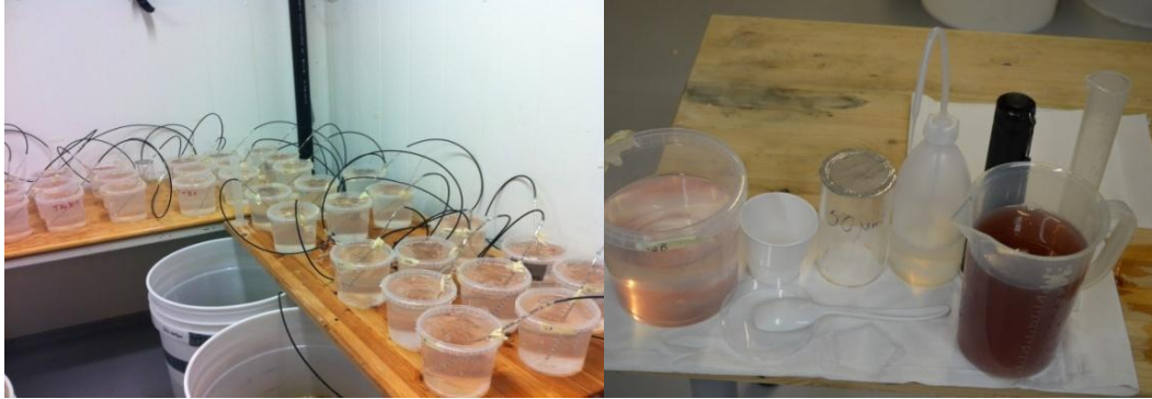
Figure 2.3. The beakers (1 L) utilized in egg production experiment (left), equipment including the egg collector with a filter sieve 50 \mu\text{m} at the bottom and for transferring of the adult copepods (right). Photo: Anh Hung Phan.
