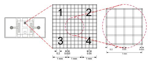
Figure B.1: Bürker counting chamber. The dimensions of the counting chamber is indicated on the figure.
