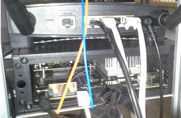
Figure 8.1: The Jetson TX1 development board, as mounted in the cyborg
