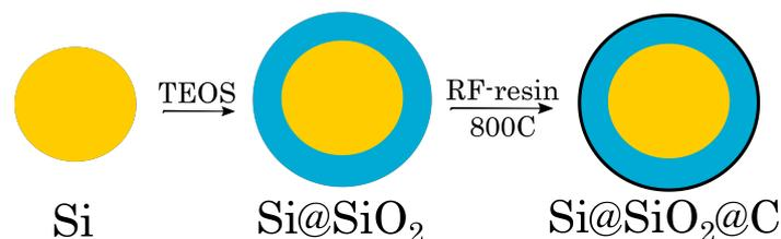
**Figure 1.2:** Producing a double core-shell particle by oxide and carbon coating.
