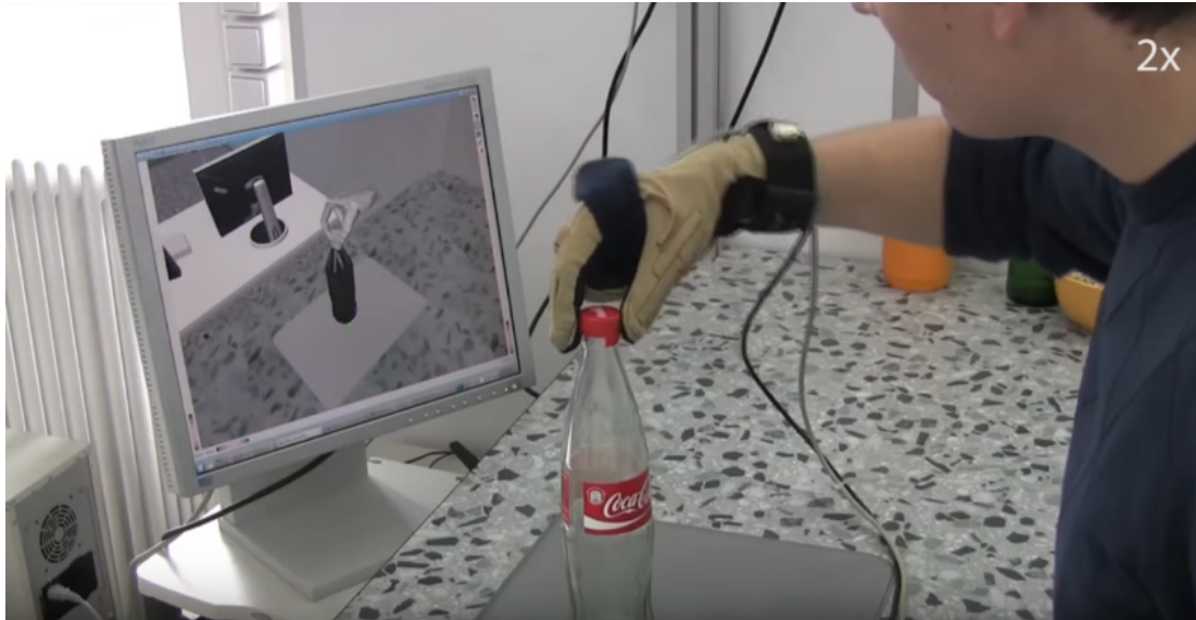
Figure 3.7: Mocap programming by example for how to open a cap on a coke bottle source( https://www.youtube.com/watch?v=jWYkzLSNmuc )
