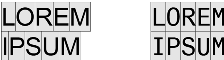
Figure 3.3: Text with a variable-width font on the left, and a monospace type font on the right
