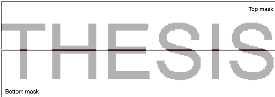
Figure 1.5: Illustration of a word with a signature with a height of one pixel
