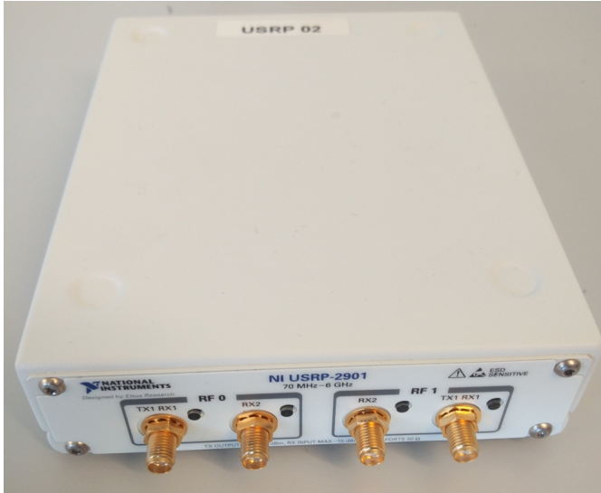
Figure 3.1: NI USRP-2901 software-defined radio
