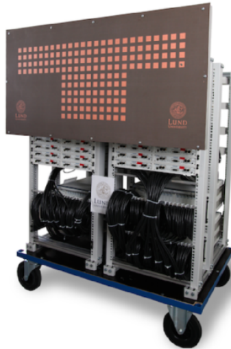
Figure 3.5: LuMaMi testbed at Lund University [15]
