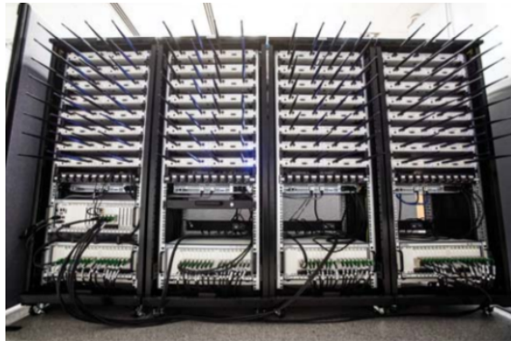
Figure 3.6: Massive MIMO 128-antenna testbed at UoB [1]
