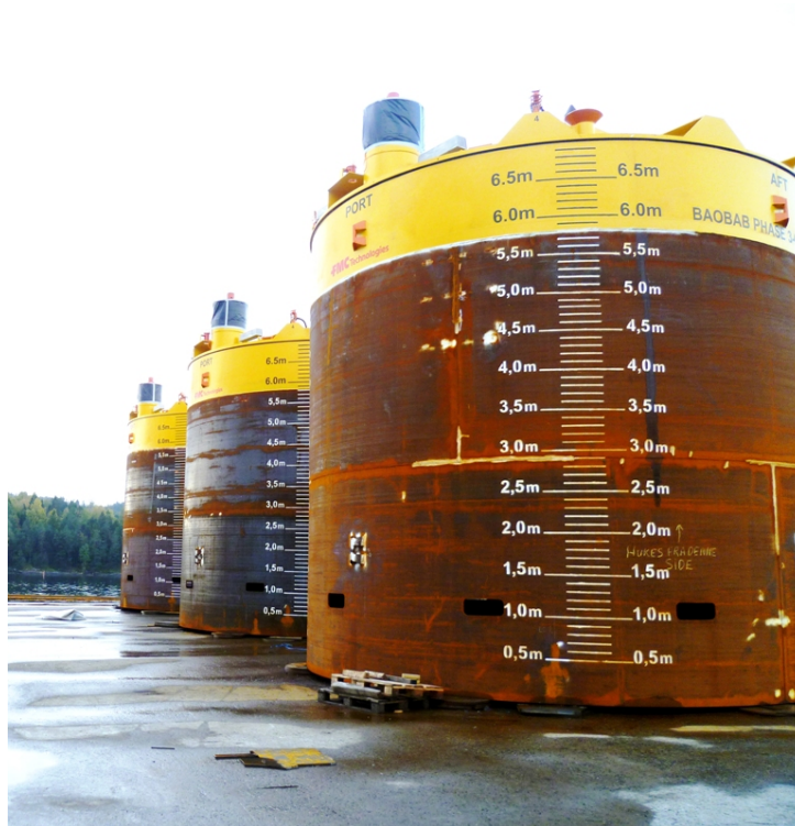
Figure 2.1: Several suction anchors lined up, each with a height of ca. 6.5 meters [16].
