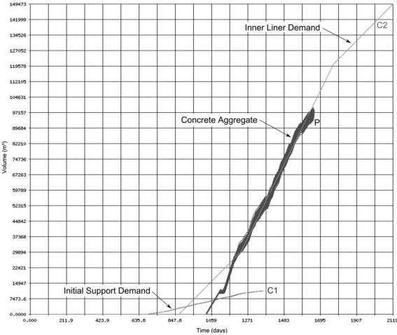
Figure 2-45: Concrete aggregate consumption through a four-year tunnel project versus the self-produced concrete aggregate. Grey area represents 100 different simulations which are based on uncertainties as evading geological conditions [23]. Self-supply of concrete aggregates is obtained 424 days after concrete consumption starts.
