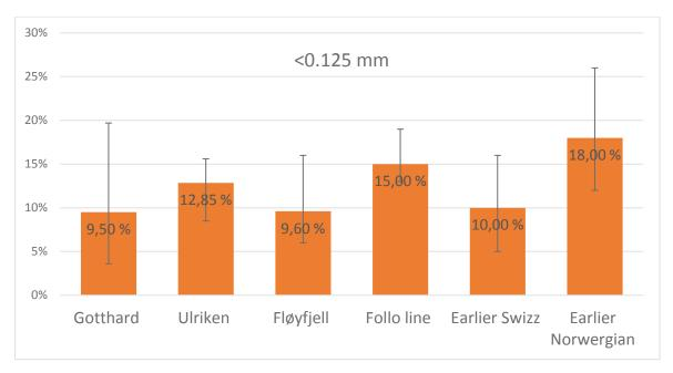
Figure 4-3: PSDs from various TBM projects and their average content of what is below the 0.125 mm sieve. The average is 11.8%.
