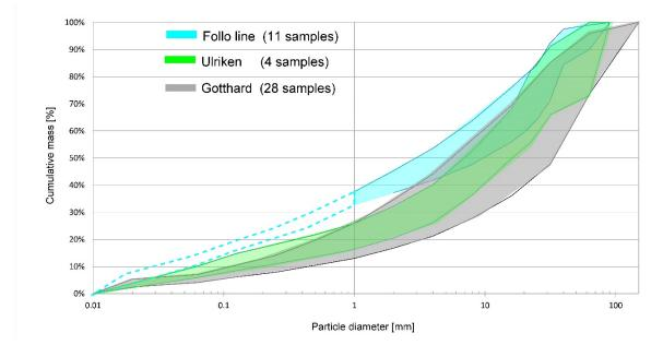
Figure 4-1: Follo line, Ulriken and Gotthard compared on its normalized PSDs, the extremes are removed. Follo line: Predicted content below 1 mm is marked with dotted lines due to missing data.
