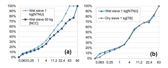
Figure 4-6: Proving differences in the use of wet and dry sieving technique and the amount used (kg) Left: T3, Right: T1.
