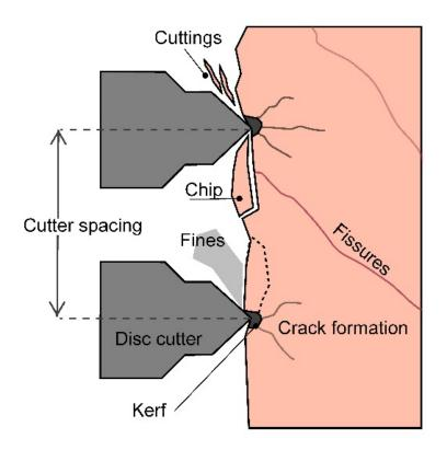
Figure 2-3: Schematic of the excavation mechanisms at the TBMs cutterhead [50].
