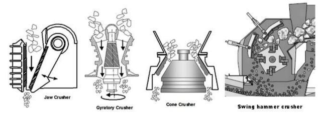
Figure 2-11: Illustration of crusher types which potentially be used in processing TBM spoil [34].
