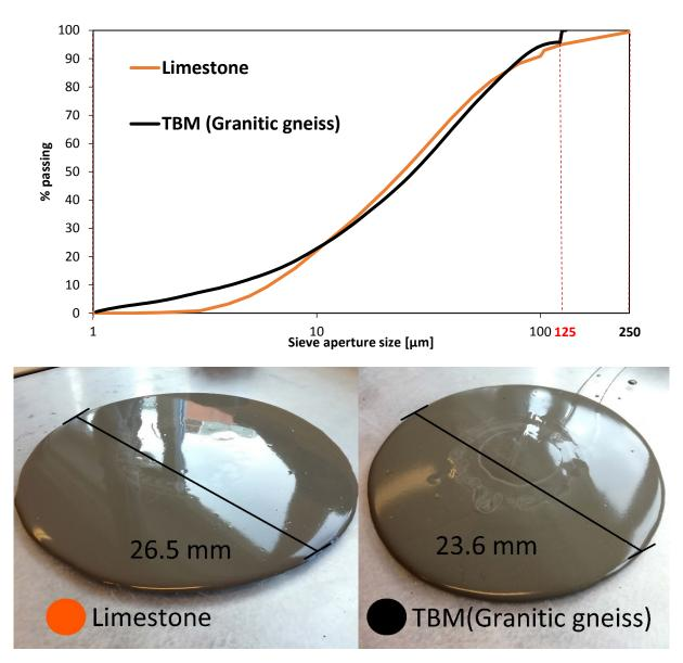
Figure 4-13: Comparing the most similar mini-slump values between the limestone and the TBM filler (T0 vs T1).
