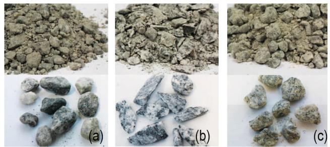
Figure 1-3: Three different 0/8 fractions from Norway. (a) The most wanted: glacifluvial originated sand, (b) low quality crushed aggregates. (c) Crushed aggregates processed through a VSI, producing a product in close resemblance to the glacifluvial sand
