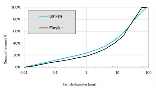
Figure 4-4: Comparing the average of PSDs from TBM projects Ulriken and Fløyfjell.
