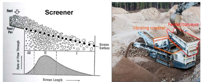
Figure 2-12: Left: Basic concept of screening through stratification and separating the feed into three fractions with a rapid separation of fines. Right, Showing Metso Scalping vibrating screener separating material into 3 different fractions [58].
