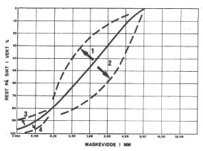
Figure 2-22: possible changes to a PSD 0-8 mm fraction[72].
