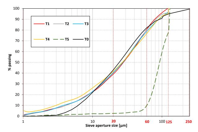
Figure 4-9: PSD of the TBM fillers from Ulriken and Follo line. The raw unprocessed TBM spoil show minor differences. It was not possible to create an identical PSD to the TBM spoil
