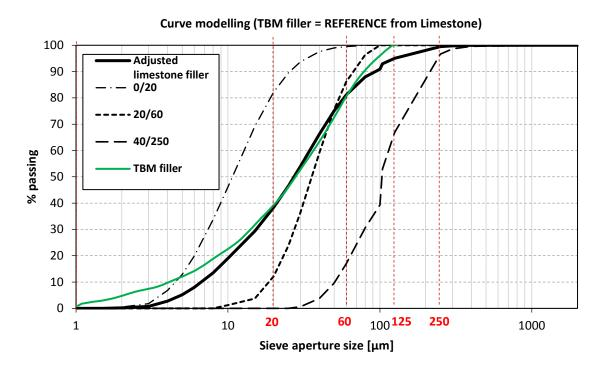
Figure 3-6: Curve modelling of limestone filler to mimic the TBM fillers. The curve "Adjusted" is a combination of 0/20, 20/60 and  $40/250 \mu$ m in the ratio 47, 38, 15% respectfully.
