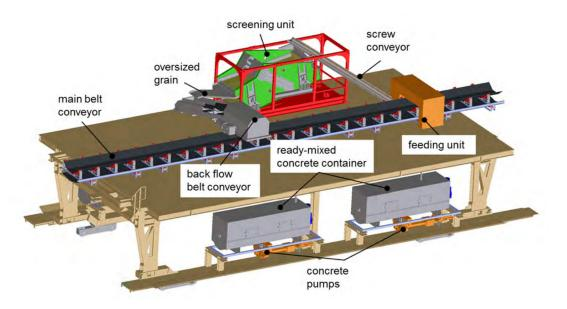
Figure 8-1: Opposite view of, now showing ready-mix concrete containers and pumps.
