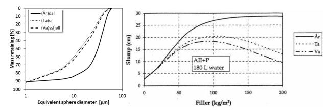
Figure 2-27: Crushed sands (Ta and Va) and natural sand (År) show increased flowability when filler amount is increased in the matrix until 100 kg/m<sup>3</sup>. Increasing the amounts above this limit reduces flowability of those concrete mixes, though the natural sand upholds a good flowability regardless. An explanation to the differences are seen in the differences in PSD in the filler fraction (<0.063 mm) [79].
