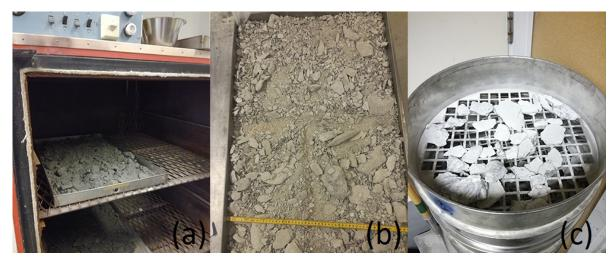
Figure 3-4: (a) Drying TBM spoil at 105 °C. (b) Reducing sample by quartering for further dry sieving. (c) Dry sieving of TBM spoil.
