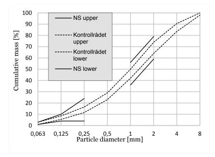
Figure 2-24: boundary conditions set for 0/8 mm natural sand.
