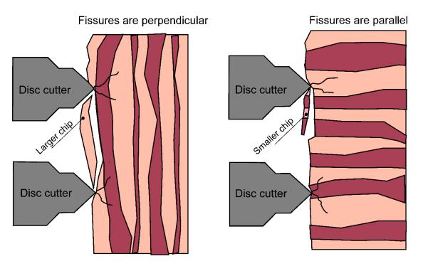
Figure 2-4: Anisotropy in relation to the cutter face angle will impact the spoil properties. Tunnelling perpendicular to the direction of fissure direction tends to generate larger and more elongated chips [28].
