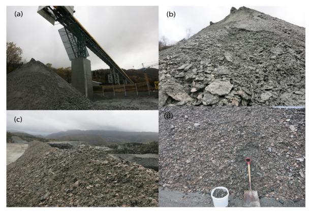
Figure 3-1: (a,b) Spoil from the TBM transported by conveyer belt, trucks would arrive based on the drilling rate that given day. (c,d) On top of one of the "mountains" of TBM spoil at NCC Ytre Arna gravel works, collecting a sample.
