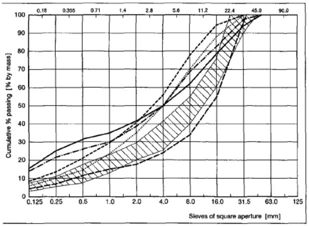
Fig. 1 – Particle size distribution of the 5 TBM materials (shaded area within SIA standard 162, art. 5, 14, 24; Fuller).
