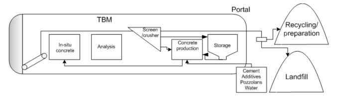
Figure 2-38: Illustrating the main procedures in the strategic plan for an automation of spoil processing [53].
