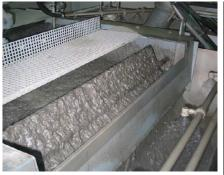
Figure 2-17: Large scale flotation was applied at the AlpTransit projects, removing the mica content in the TBM spoil fractions  $63/125 \ \mu m$  and  $125/250 \ \mu m$ [53].
