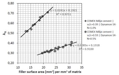
Figure 2-29: Two concrete receipts with w/c=0.39 and w/c=0.59. Both mixes have been altered with varying fillers and varying filler/cement ratio. The prominent flow impactor is nonetheless the surface area of the filler. [82]
