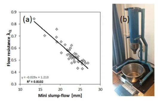
Figure 2-31: (a) The correlation between mini slump-flow and the flow resistance measurement  $\lambda_Q$  [84]. (b) The FlowCyl apparatus, the weight measurement frequency is set to 2/sec.
