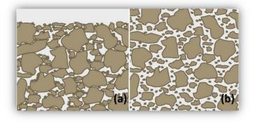
Figure 2-25: (a) Aggregates packing with no interference. (b) Aggregates dispersed and lubricated by the matrix[73].
