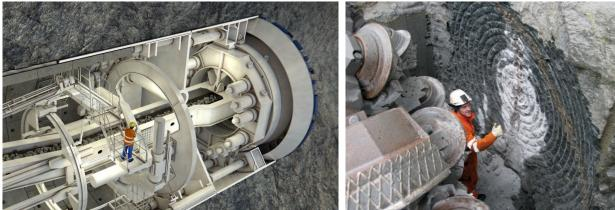
Figure 2-1 Left: Illustration of a double shield TBM[42]. Right: An engineer is inspecting the tunnel at a project at Faroe Island in 2010. The spacing and penetration is visible in the rock face [43].
