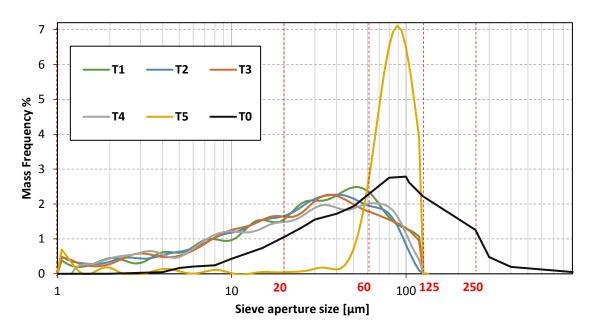
Figure 4-10: The mass frequency of the different TBM materials. Minor variation in the frequency of the 4 TBM spoils. The processed 0/8 mm follo line aggregate(T5) do show high occurrence between 60-125  $\mu$ m. This can be explained by the reduction of fines with the cyclone placed at Åsland.
