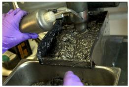
Figure 2-18: Laboratory setup for the froth flotation. The picture shows a laboratorist adding a "frother" to reduce the tension of the pulp(bubbels) and collecting the wanted/unwanted minerals at the surface [63].
