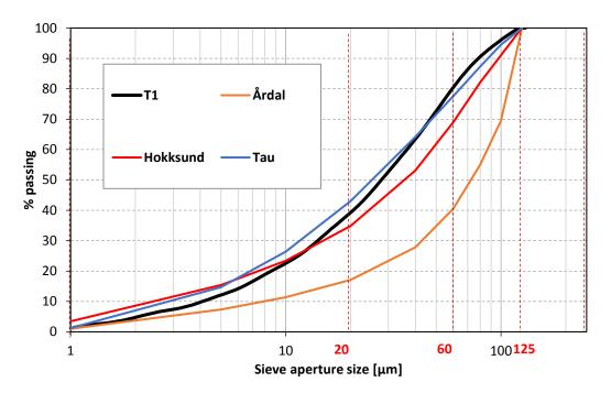
Figure 4-12: The crushed rock by either cone crusher, VSI or TBM cutter head shows similar PSD below 0.125 mm. The natural Årdal shows a coarser PSD.
