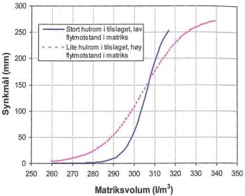
Figure 2-26: The correlation between slump value and matrix volume. Until slump values of 150 mm the most efficient slump is achieved with the so-called particle dominated mix. Slump values above 150 mm will be ruled by the matrix as it's volume is large enough to increase the spacing between aggregates [77].
