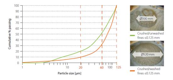
Figure 2-28: Two similar concrete recipes with w/c=0.5. Green line is unwashed filler and orange is washed filler. The differences in PSD in the filler fraction is seen to have significant impact on slump value in the fresh state. [37]
