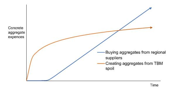
Figure 5-2: Concrete aggregate expenses in a TBM project. Illustrating the economic potential of investing in a processing facility for spoil utilization. After a certain period, the investment cost of the facility will pay off in terms of reduced need for external aggregates. The initial growth by the orange curve are illustrating the investment of a processing facility[18].
