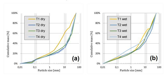
Figure 4-7: 1 kg PSD measurements of the TBM spoil, wet and dry sieved technique applied.
