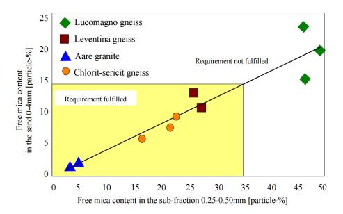
Figure 2-20: Correlation between free mica content in 0/4 mm and 0.25/0.5 mm fraction. Yellow zone represents a sand which have fulfilled B30/40 concrete [33].
