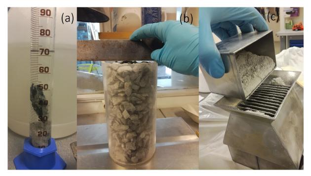
Figure 3-5: (a) Density measurement of cuttings by submerging in water. (b) Packing grade measurement. (c) Splitting of filler in preparation for the SediGraph.
