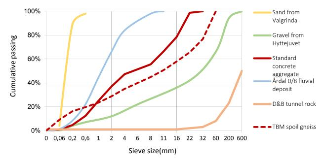
Figure 1-2: The PSDs illustrates the TBM spoils close resemblance to concrete aggregates in comparison to other granular sources.
