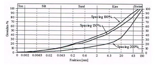
Figure 2-8:Increasing spacing between disc cutters results in a coarser PSD [53].
