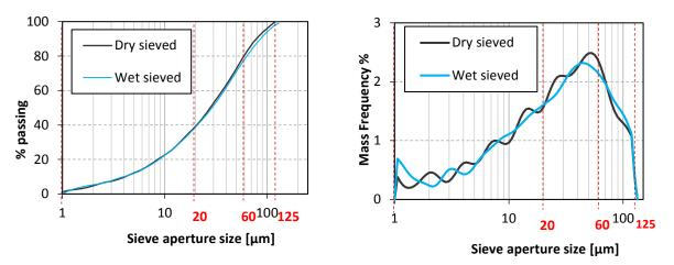
Figure 4-11: TBM spoil(T1) has been dry sieved and wet sieved. Afterwards has both samples has been extracted on the fraction <0.125 mm and been analyzed with the X-ray sedimentation. Minor differences in the PSD is noticeable.
