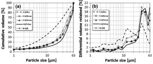
Figure 2-30: (a) PSD measurements with X-ray sedimentation method. (b) presented by difference in volume [83] C-0/8-u = crushed unwashed C-0/8-nw = crushed normal wash C-0/8-hw =crushed hard wash N-0/8 = Natural
