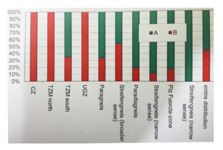
Figure 2-41: Displays the ratio of A and B material, excavated from GBT sorted in zones excavated. CZ(Clavaniev zone), TZM( Tavetsch intermediate massiv), UGZ( Urseren-Garvera zone) [55].
