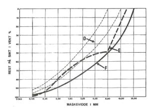
Figure 2-23: Suited PSD for different types of concrete, 0-8 mm fraction [72].
