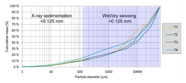
Figure 5-1: The PSDs produced can be combined. The X-ray sedimentation PSDs are not easy to differentiate at this scale.
