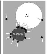
Figure2-19:Illustrating how and air bubble ascends to the surface and attaches to the hydrophobic mineral along the way (e.g. mica)[62].
