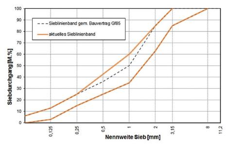
Figure 2-44: Boundary lines for the 0/8 mm fraction. The boundaries allow for high amounts below 0.125 mm [98].
