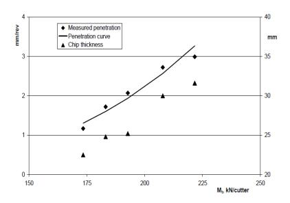
Figure 2-6: Increasing chip thickness with increasing penetration in a mica gneiss [49].
