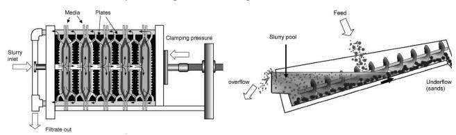
Figure 2-15: Left: dewatering of mud water with filter press( VPA) for removal of fines [62]. Right: Dewatering of coarser particles with a bottom spiral classifier [62].
