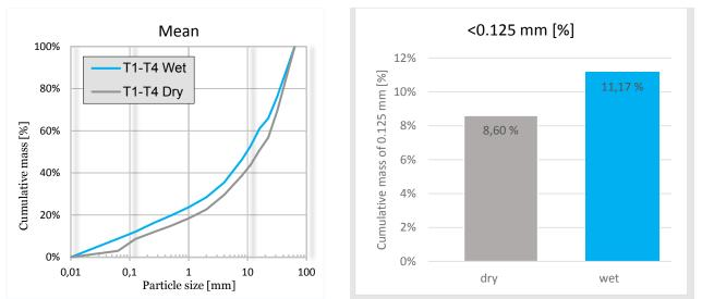
Figure 4-8: Left: Wet sieve always creates a finer PSD when compared to dry sieve. Right: T1-T4 compared on the 0.125 mm sieve
