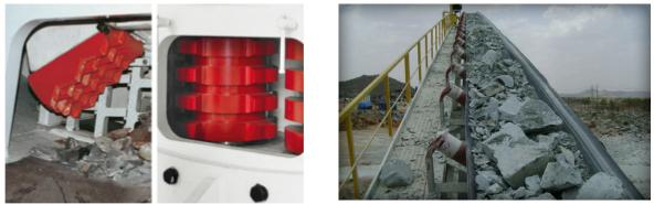
Figure 2-2: Left: Jaw or roll crusher can be installed behind the TBM shield to guarantee maximum spoil size on conveyer belts. Right: Double Shield TBM spoil transported on a conveyer belt at Alimineti Madhava Reddy Project in India [46, 47].
