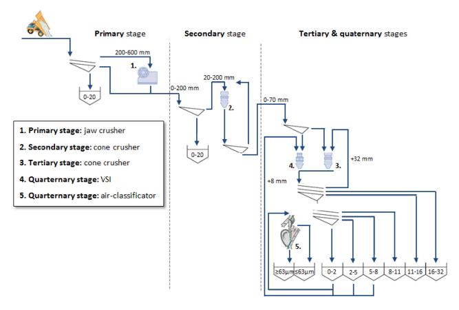
Figure 2-10: Processing of crushed sand, the quaternary stage is illustrated with a dry process, though wet processing is also possible [13].
