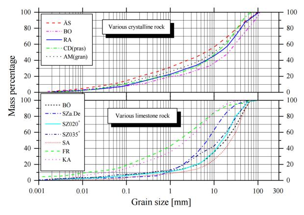
Figure 2-9: PSDs from different TBM spoils in Switzerland, sorted by crystalline or various limestone rocks [38].
