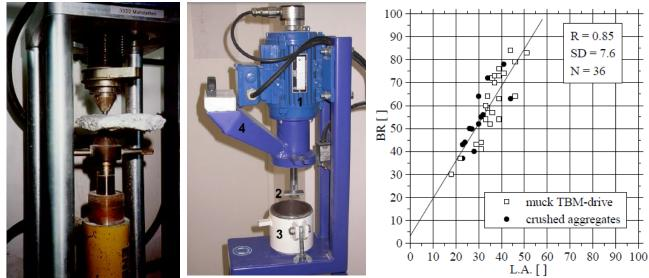
Figure 2-21: Left: Point load apparatus[33]. Middle: The LCPC apparatus measuring crushability(CR). Right: The CR correlates to the LA test on both crushed aggregates and spoil [50, 69].
