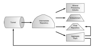
Figure 2-40:Left: general flow chart for an Swiss made approach of excavated material called TEMH( Tunnelling excavation material handling) 2012 [23, 33].
