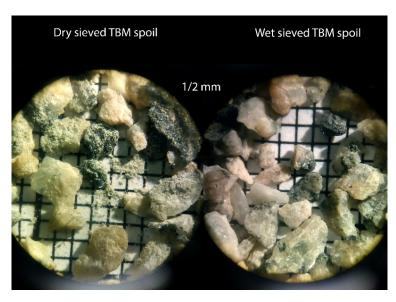
Figure 4-5: Fines have a cohesive binding to particles which stick to the dry sieved spoil. Light scraping on the dry sieved 1/2 mm fraction and finer particles fell off. Squares are 1 mm.
