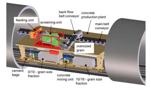
Figure 2-37: Illustrating the concept of processing TBM spoil in the "back-up" for CIP concrete. Aggregate storage, cement storage and mixing plant is not seen in the illustration.[53]
