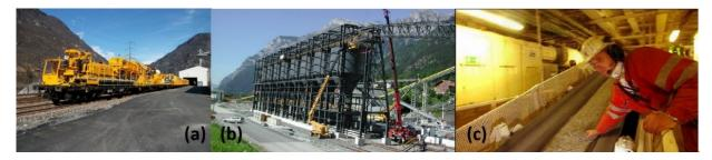
Figure 2-36: (a) The concrete batching plant train[92]. (b) Aggregate silos for the concrete train at Amsteg, (c) Inspecting aggregate quality at Amsteg aggregate plant [93].
