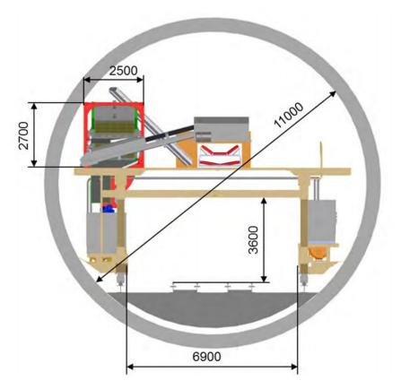
Figure 8-2: Cross-sectional view of screening unit placed inside the tunnel connected to the main conveyer belt.
