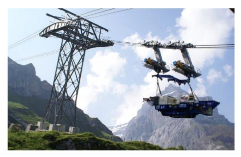
Figure 2-13: A 38 ton mobile impact crusher(swing-hammer) combined with a screening unit are being transported to the tunnel site(2500 ASL) at the Linthal-Limmern power station for the purpose of dry processing TBM spoil [61].
