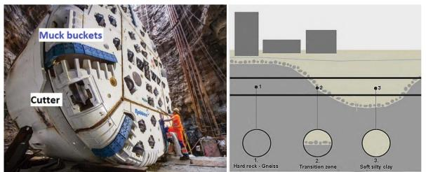
Figure 1-1: Left: Double shield TBM with 7m diameter in Ohio, USA [9]. Right: Potential geological conditions for underground tunnelling, a key parameter if the spoil is to be utilized as concrete aggregate [10].
