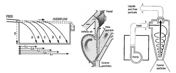
Figure 2-14: Left: Showing horizontal traveling path of falling sand particles in a classifier tank[57]. Middle: Particle path in gravitational inertial classifier[34]. Right: Creating a vortex to separate particles in a Hydrocyclone classifier [34].
