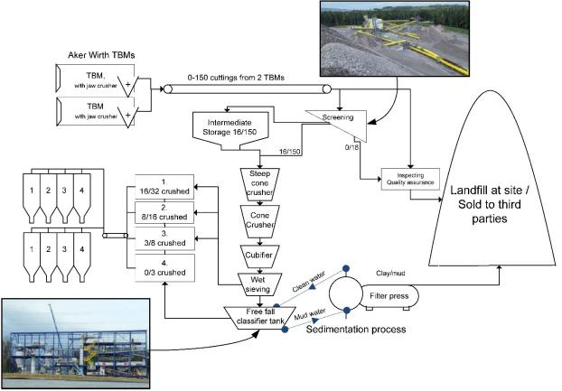
Figure 8-3: Flow diagram is based on report: Use of recycled material for segments and inner lining – first experience of on-site processing on KAT 2 [1].
