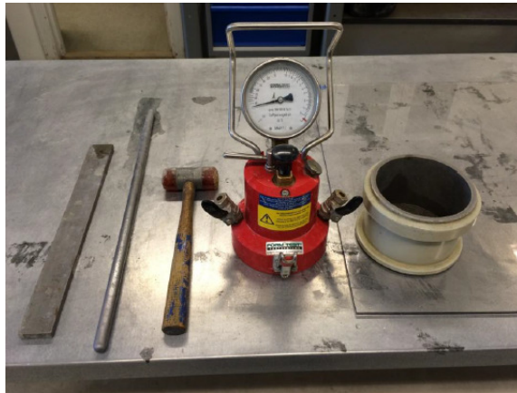
Figure 6: Picture of the pressure- and density method equipment.
