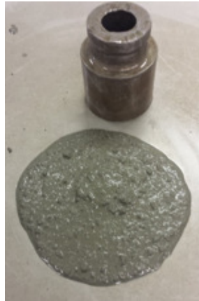
Figure 5: Slump test showing a slump of around 110 mm
