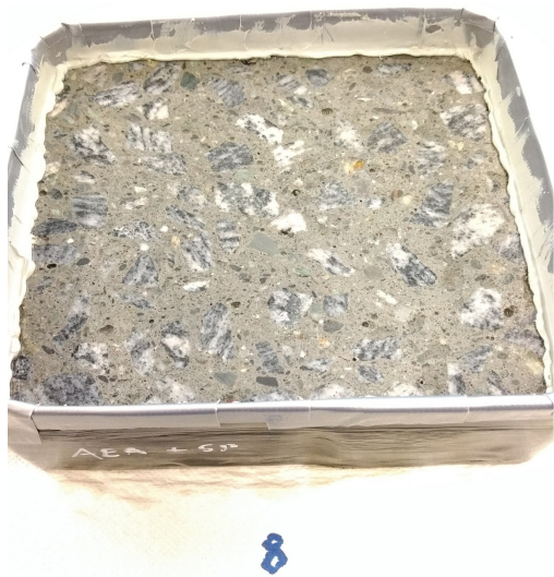
(a) Sample 8, Damages after 28 Cycles
