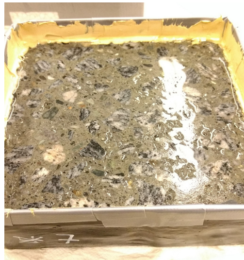
(b) Sample 7, Scaling after 28 Cycles
