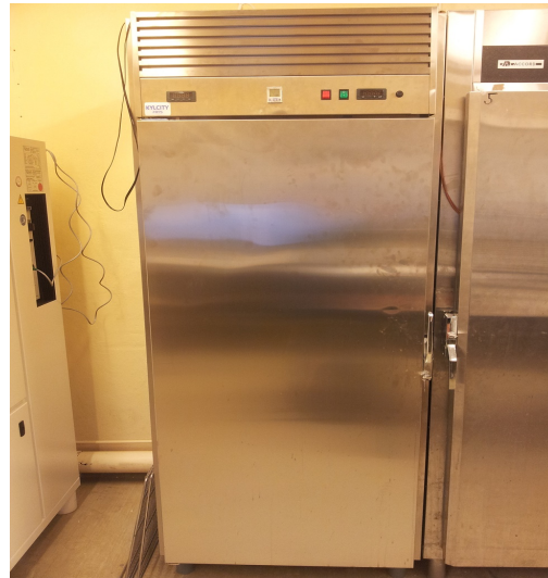
(b) KylCity freeze-thaw chamber
