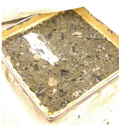
(a) Sample 7, Damages after 28 Cycles
