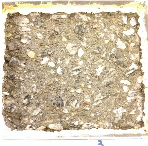
(a) Sample 2, Damages after 28 Cycles
