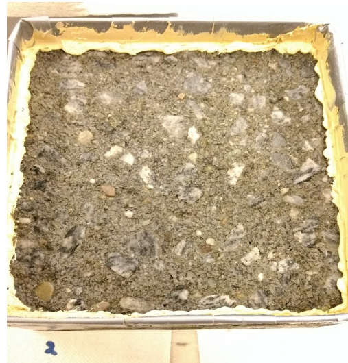
(b) Sample 2, Scaling after 28 Cycles
