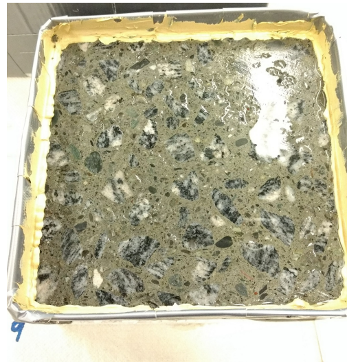
(b) Sample 9, Scaling after 28 Cycles
