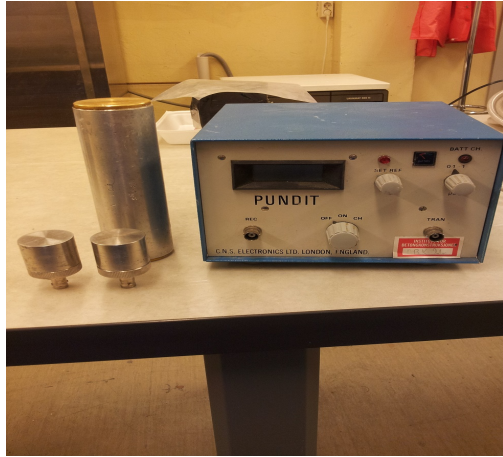
(a) UPV Equipment
