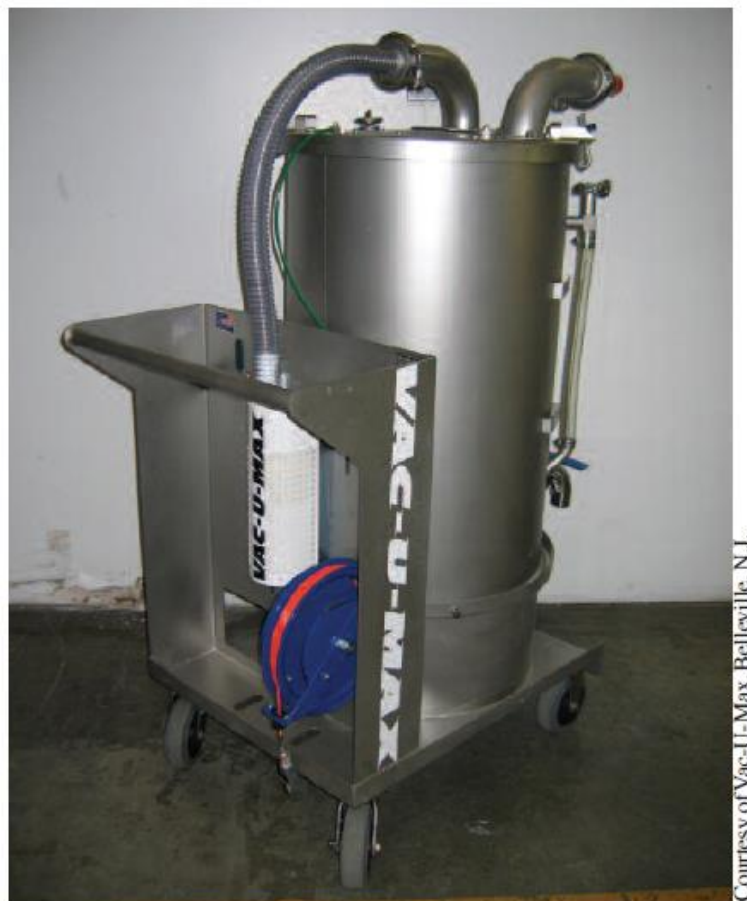
Figure 18: Submerged- (or liquid-) recovery portable vacuum cleaner.
