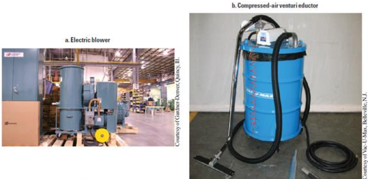
Figure 17: Vacuum producers for portable vacuum cleaner.
