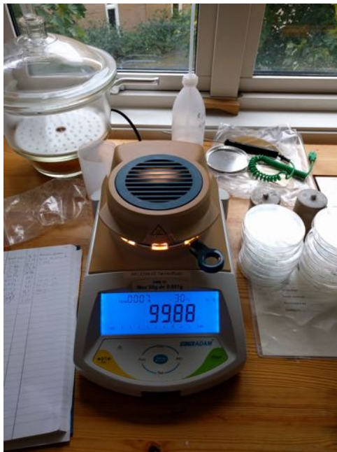
(b) Dy fibre concentration measuring
