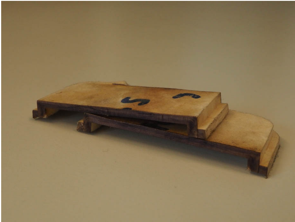
Figure 3.4: The laser cut edge of a TMP sample
