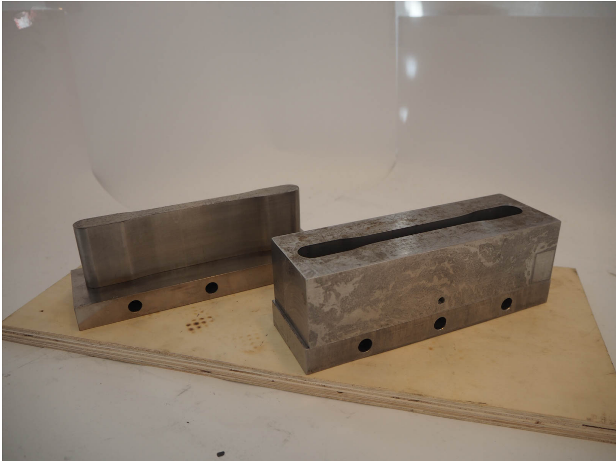
Figure 3.2: Spark eroded steel mould assembled
