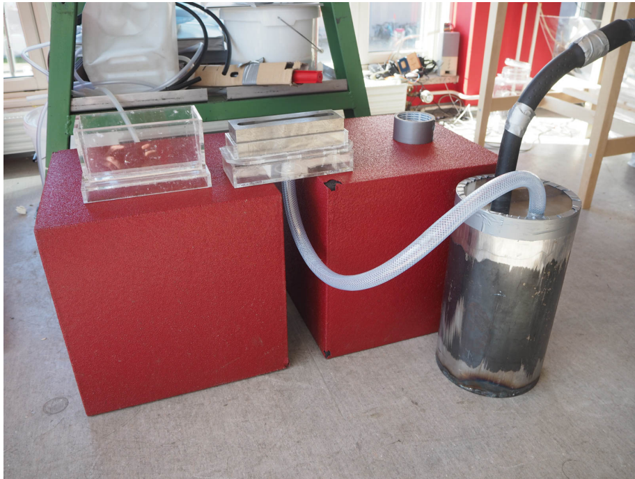
Figure 5.1: Pre-filtering setup: The female part of the mould, with the bottom detached, is inserted into the socket of the acrylic vacuum chamber which is connected to the steel chamber. The acrylic funnel is then placed on top of the mould and the pulp is poured into the funnel and the vacuum is turned on.
