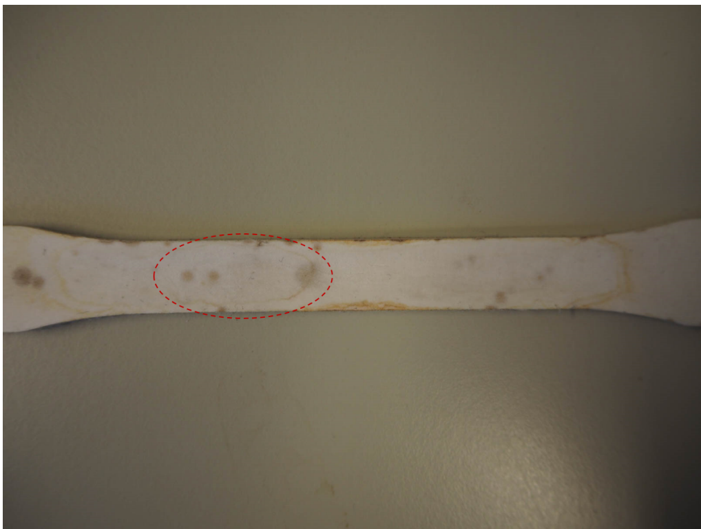
Figure 4.19: Detail picture of moulded Kraft sample with 2% MFC content. The dotted circle shows the wet pocket that has emerged inside the already affected narrow section.
