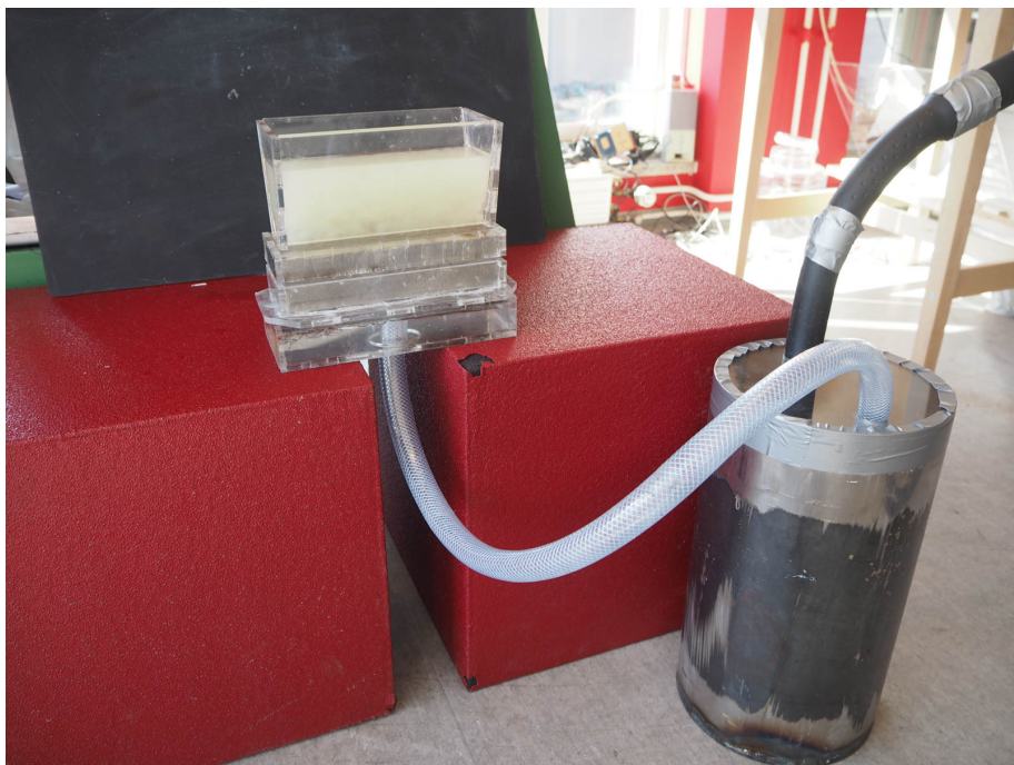
Figure 5.2: Pulp filtering: This is what the setup looks like after the pulp has been poured into the funnel and the filtering has begun.
