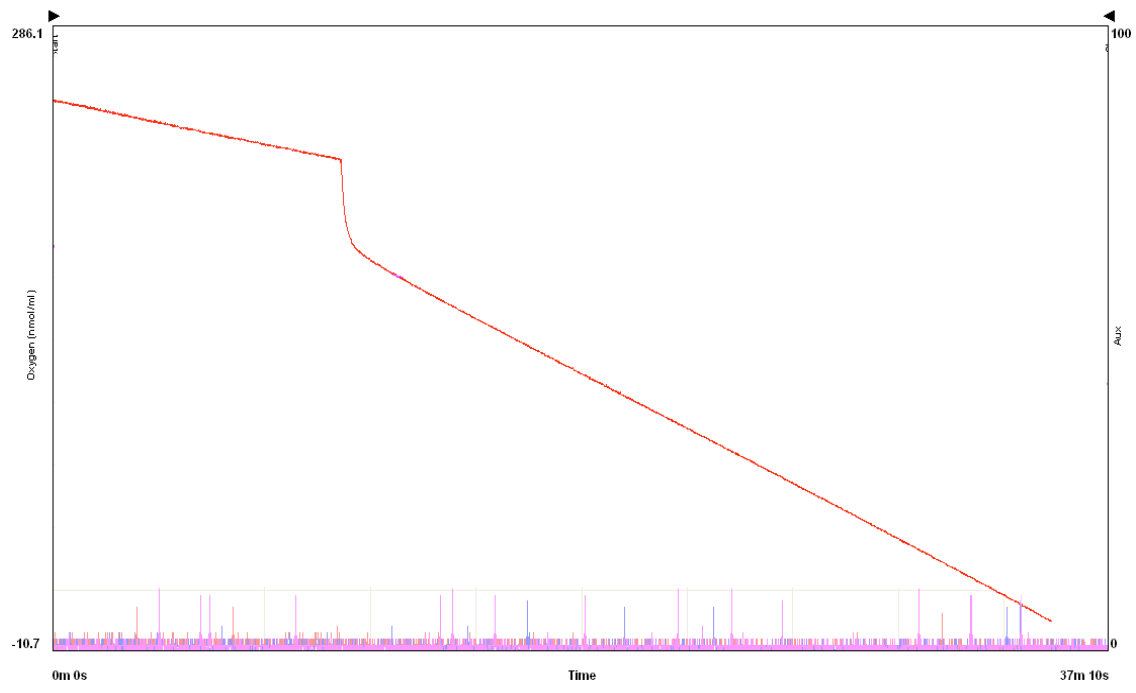
Figure 30: The kinetics of oxidation of 0.6% liposomes induced by \text{Fe}^{2+} ( 50 \mu\text{M} ). 5 mM MES buffer was used as solvent.
