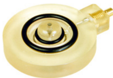
Figure 18: Electrode disc (Mozuraityte, Rustad et al. 2006).
