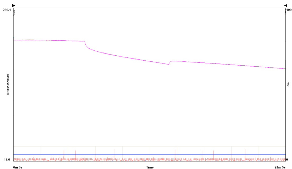
Figure 19: Oxygen uptake rate measurement by polarographic oxygen electrode.
