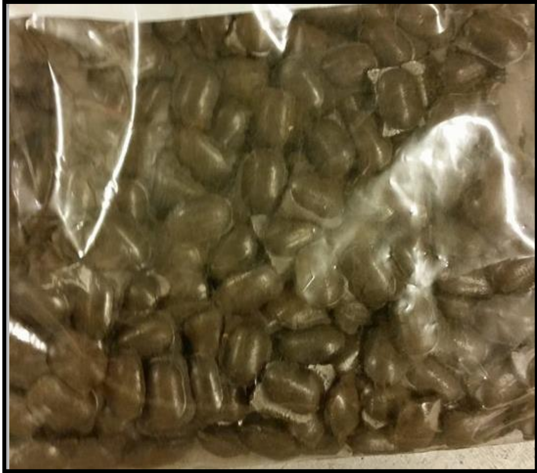
Figure 19: Picture of the briquettes produced with Briketta from the 8wt% lignosulfonate batch.
