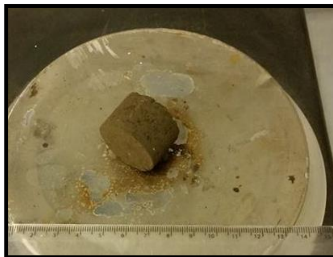
Figure 15: Briquette made with 6wt% Lignosulfonate. Diameter 30 mm, height 21 mm
