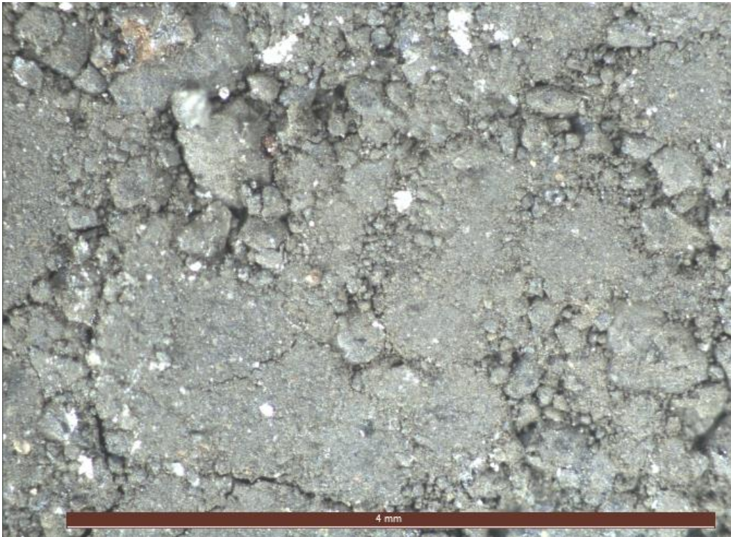
Figure 50: Macro image 8wt% lignosulfonate, 16x
