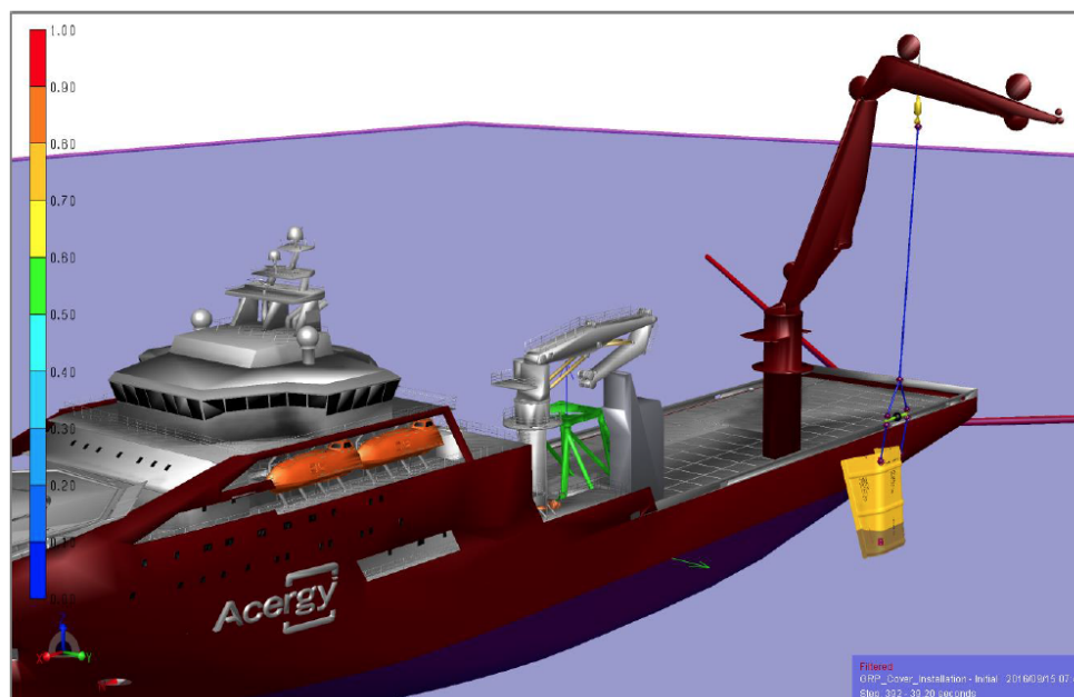
Figure 10.2: Vessel lifting cover in vertical direction (Statoil, 2015)
