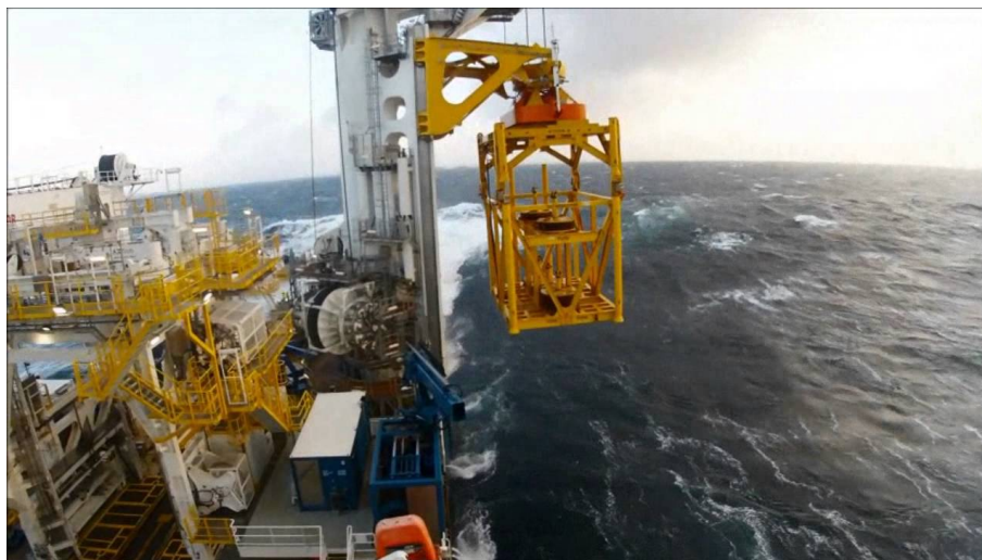
Figure 3.5: A test of a Special Handling System on board the North Sea Giant outside Sandnessjøen (AxTech, 2017b)
