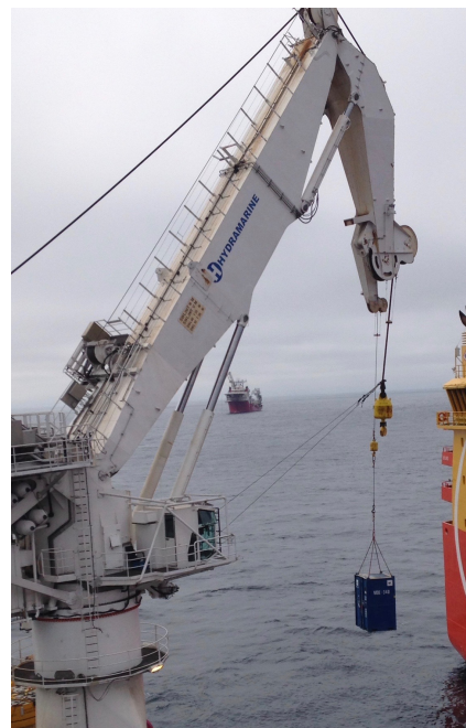
Figure 3.3: Crane operation over side
