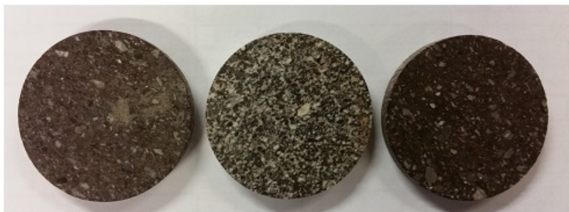
Figure 8.1: Samples prepared as disks for swelling pressure test. Left: PK 34+405, Middle: PK 36+555, Right: PK 37+060.
