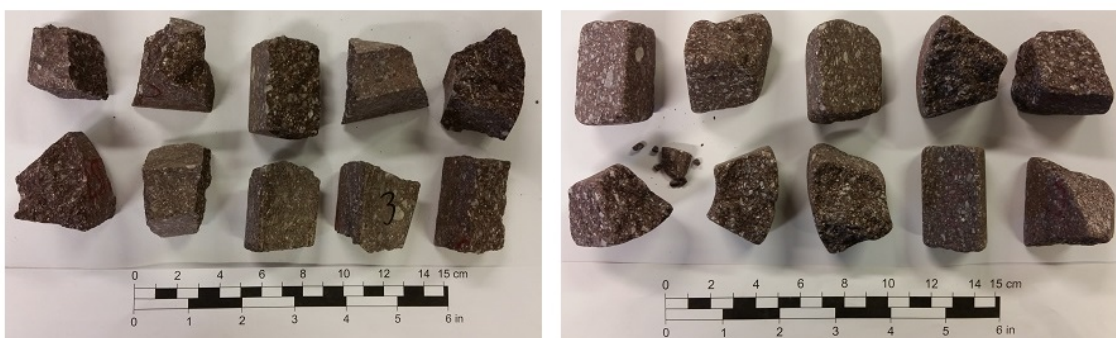
Figure 8.9: PK 37+060, samples before and after 4 cycles of slake durability test.
