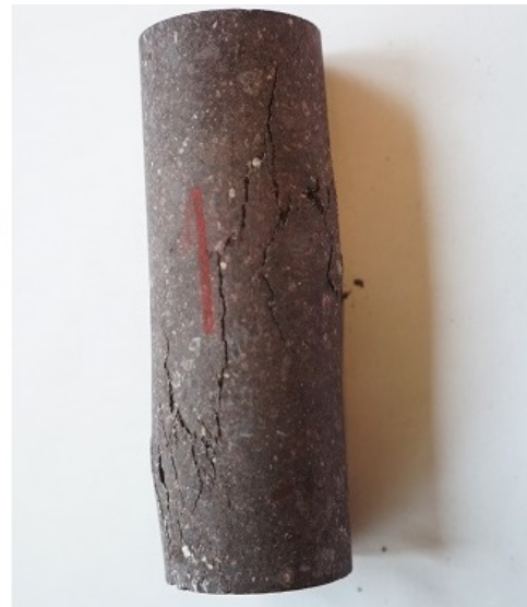
Figure 8.7: Result from uniaxial compressive test. Axial stress plotted against axial and radial strain. Image of PK 34+405 showing the failure mode, which appears to be shear failure.
