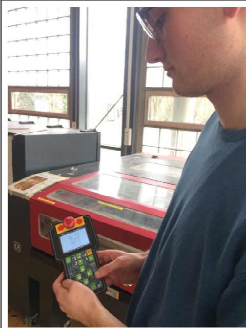
Figure 4.4: Industrial design. The handheld controller is used for setting the starting position and running the pre-made jobs from a server.
