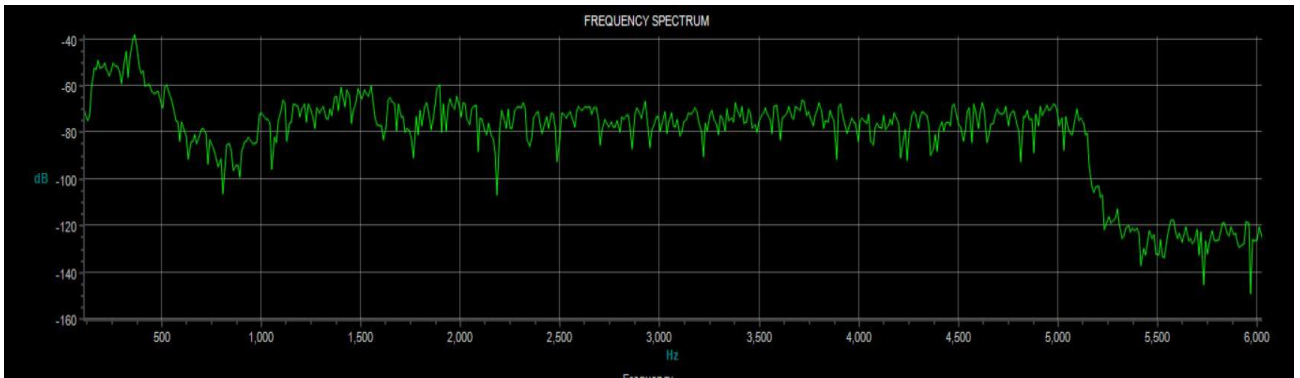
Figure 9: Laser Cutter frequency spectrum from only 0 to 6 000 Hz.
