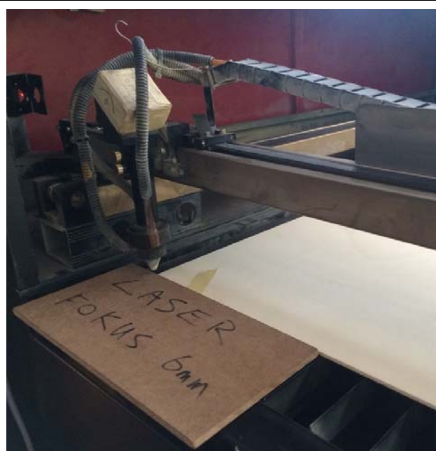
Figure 4.5: Industrial design. A 6mm thick MDF-sheet is used for setting the correct laser cutter height when cutting 1mm cardboard. Misfocus could lead to poor surface quality or start a fire.
