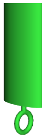
Figure 3.4: Close-up of profiled aluminum rod with the screw eye inserted at the bottom.
