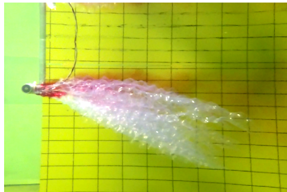
(c) The undulate blades suppress the alternating vortex shedding.
