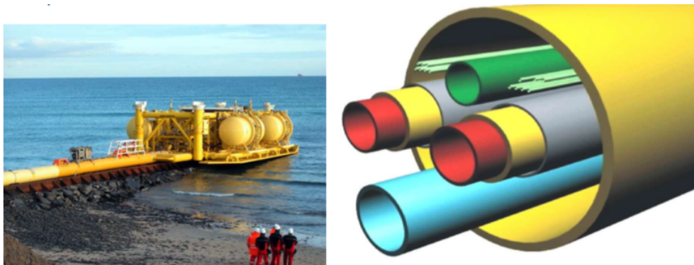
Figure 2.9: Towhead and schematic of cross section of bundle. Subsea 7 (2012)
